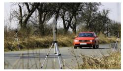
The measurement setup of noise emission of passing road vehicles is defined by international standards. Also environmental conditions like ground temperature is is considered in the standards. For different categories (two-wheelers, passenger cars, LCV, HCV, trucks, busses etc) different procedures exist.
