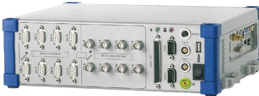
The CAPS-STD system (DEWE-211-CAPS-16) shown in the picture is typically equipped with 16 analogue input channels, 16 digital input channels, 2 counter channels and two CAN interfaces. It also offers external channel expansion via the integrated EPAD2 connector. Thanks to its integrated solid state hard drive it ensures data safety even in rough environments.
