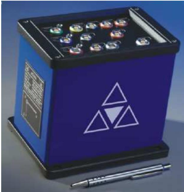
The ADMA gyro system was especially developed for dynamic testing of vehicles. The ADMA-G continuously measures both the acceleration and position in all three axes and the pitch, roll and heading angle of a moving vehicle. The system can also be used for the dynamic calculation of speed. The ADMA-G is the sophisticated ADMA version with an integrated GPS receiver for highly accurate measurements.
