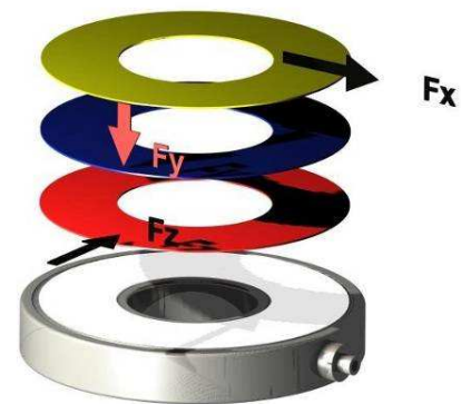
Figure 8: set-up [configuration] of a three-component force sensor
