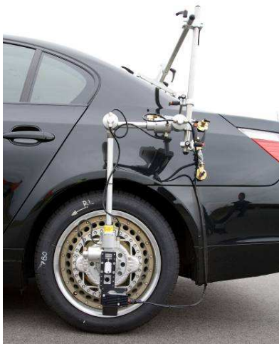
Figure 7: 6-component vehicle wheel measurement wheel at the rear axle
