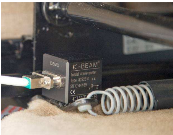
Figure 10: seat rail accelerometer
