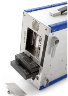
DEWE-3020 with opened battery compartment
