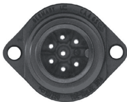
7-pin AMPFLEX connector (male)
