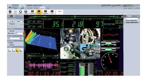
The FG-VIDEO-4-x frame grabber cards are fully supported in DEWESoft 7 and offer four parallel powerful video interfaces. This way four color PAL/NTSC cameras can be added to the measurement system. Each camera can run at up to 30 frames per second.
