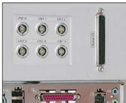
Built-in digital I/O and counter/encoder connectors (option)
