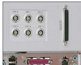
Built-in digital I/O and counter/encoder connectors (option)
