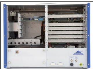
Rugged guides for full-size cards and a fixing bar hold all installed cards in place safely.
