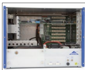
DEWE-2608 6 slots full length and 1 slot half length
