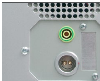
Option 800-DC-12V Internal 9 .. 18 V DC power supply including external AC adaptor.
