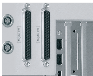
Built-in digital I/O and counter/encoder connectors
