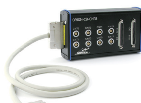
BOX-ORION-CB-CNT8 for easy sensor connection
