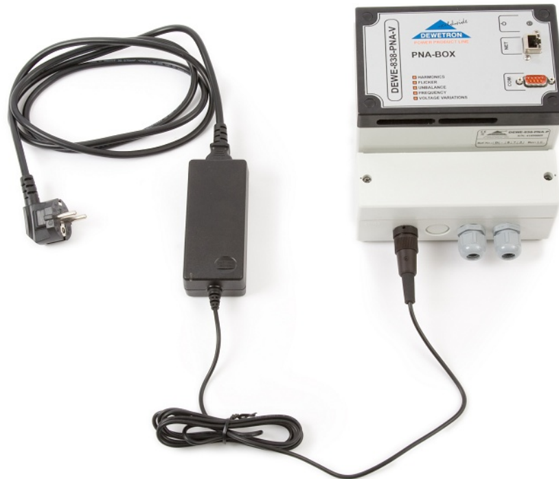
DEWE-838-PNA connected to the power supply
