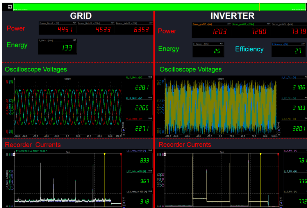
Picture 1: Example Screen of the software for an Inverter-measurement powered by the grid (3-phase)
