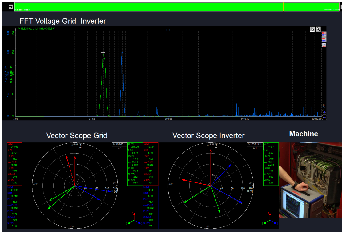
Picture 4: FFT and vector scope of the inverter and the grid
