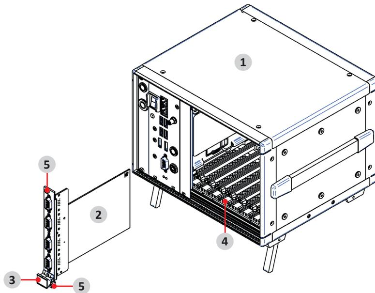
Fig. 5: Installing a TRION module (symbolic image)
