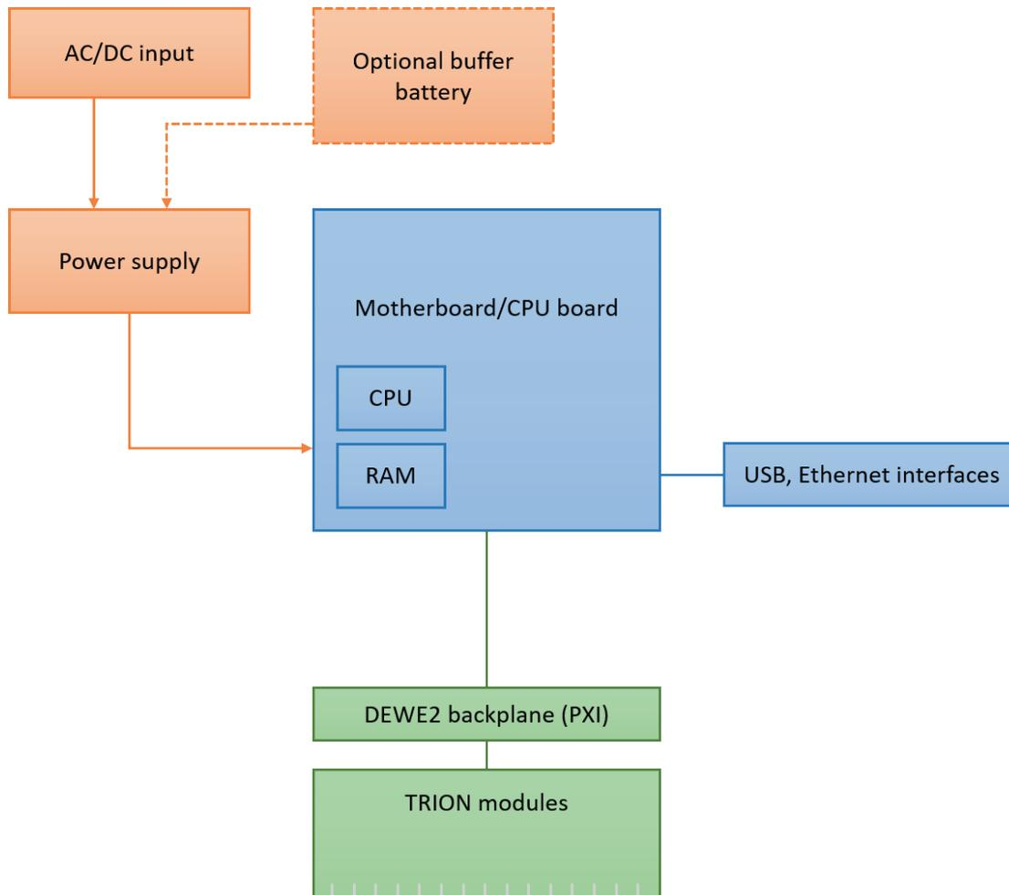
Fig. 2: Block diagram of the internal signal processing
