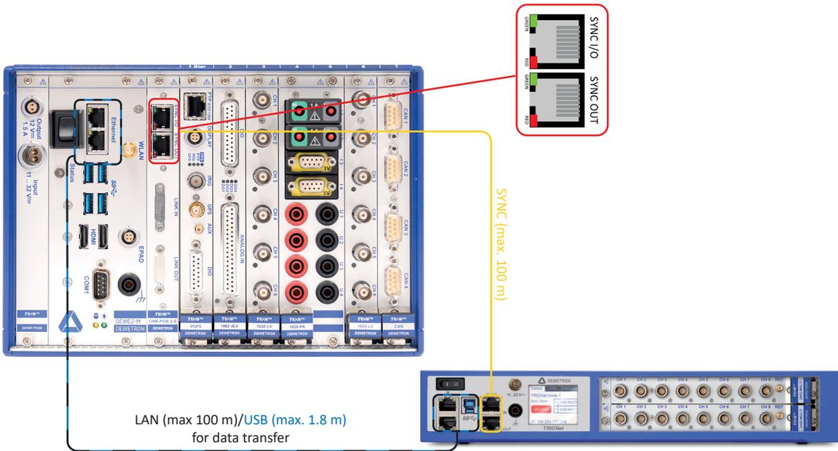
Fig. 7: Channel expansion with TRIONet
