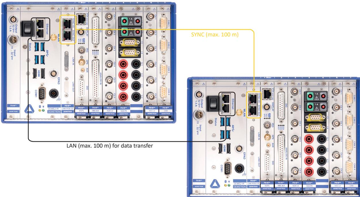
Fig. 8: Network with multiple systems
