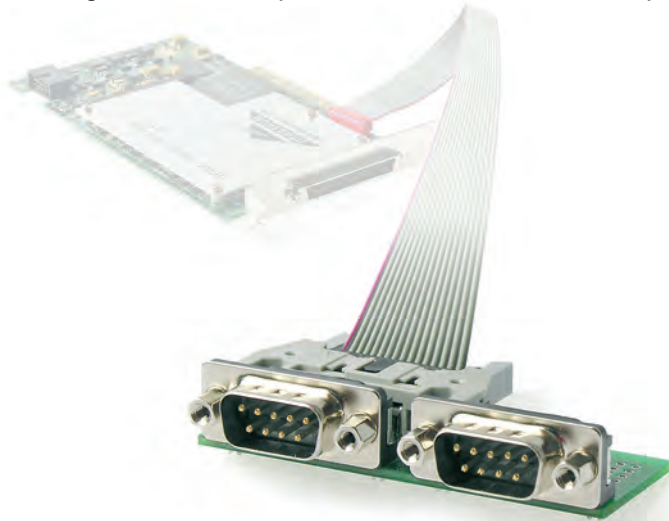
Two 9-pin SUB-D connectors prepared to be mounted inside systems
