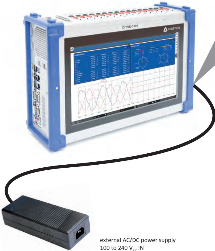
DEWE-3300 with option '3300-PS-DC-200' and included external AC/DC power supply
