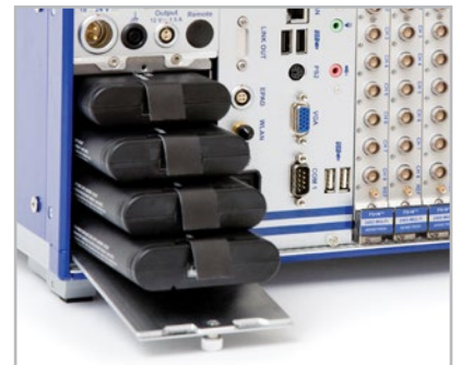
4 slots for hot-swappable batteries (option DW2-PS-BAT)
