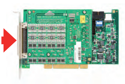
ORION base board connector (68-pin amplimite series)
