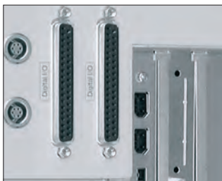
Built-in digital I/O and counter/encoder connectors
