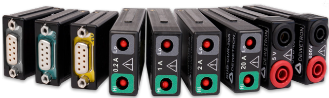
Fig. 136: Available TRION sub-modules
