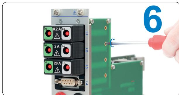
Secure the replaced sub-module with the torx screw (M2x4, TX6). Max. torque: 0.2 Nm
