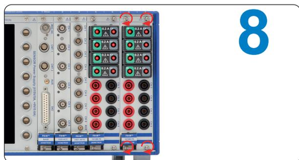
Pull up the injector/ejector handle to latch the module. Tighten the screws at the top and bottom of the TRION-1820-POWER-4 module front panel (4x) to secure the module.
