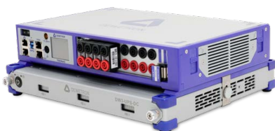
TRIONet3 with DW3-UPS-DC battery pack for independent power supply
