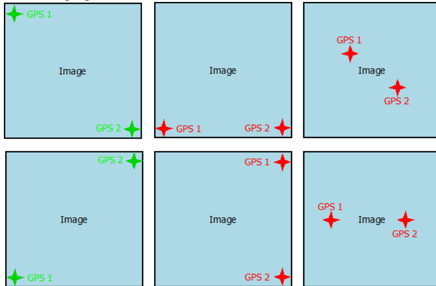
Figure 3-4: Good (left) and bad examples (middle, right) for selecting GNSS coordinates on the background image
