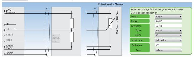
Fig. 83: Half bridge or Potentiometer 5 wire sensor connection
