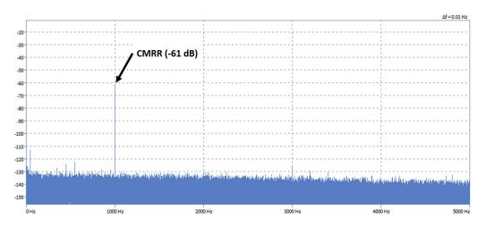
Fig. 227: Measurement of CMRR in FFT chart of TRION-1620-ACC (>2 V range @ 1 kHz)
