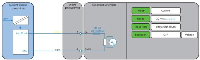
Fig. 52: Current measurement (with externally powered transmitter
