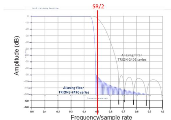
Fig. 79: Transfer function of aliasing filter at 100 kS/s
