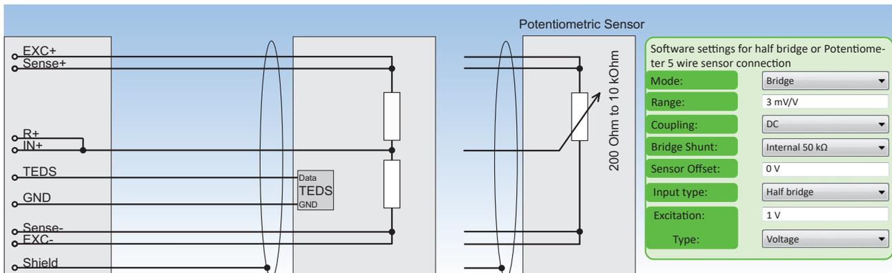
Fig. 123: Half bridge or Potentiometer 5 wire sensor connection
