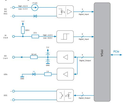
Fig. 43: Digital block diagram
