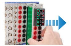
4. Loosen the torx screw (M2x4, TX6) which secures the sub-module of the channel you want to replace.
