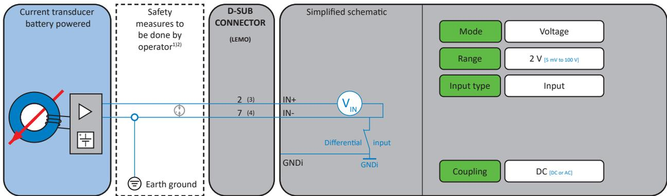
Fig. 31: Current transducer with voltage output
