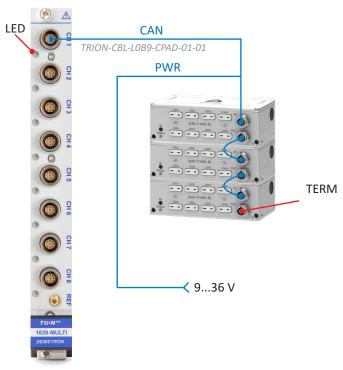
Fig. 76: Connecting XR modules to the TRION(3)-18xx-MULTI
