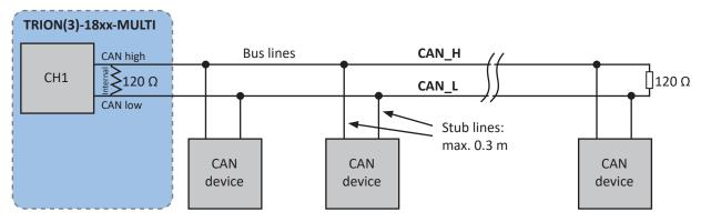
Fig. 73: CAN bus connection
