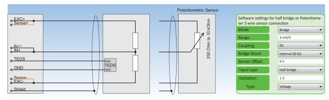
Fig. 110: Half bridge or Potentiometer 3 wire sensor connection
