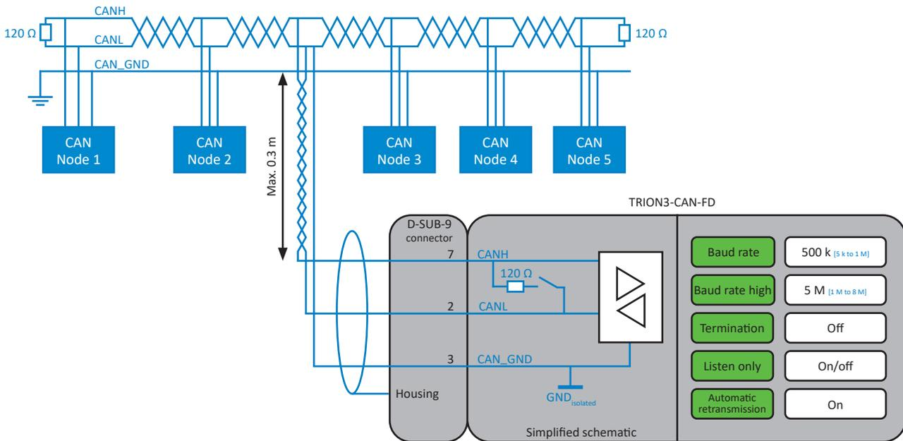
Fig. 218: Analyzing or monitoring a CAN bus
