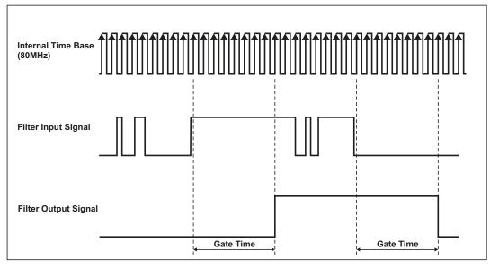
Fig. 193: Input signal with jitter
