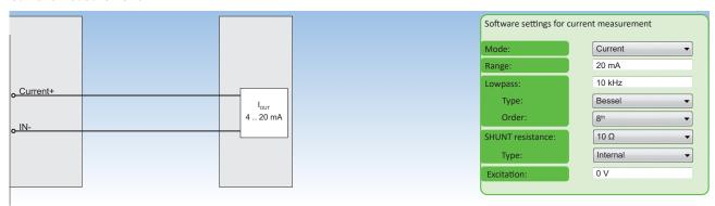
Fig. 39: Current measurement
