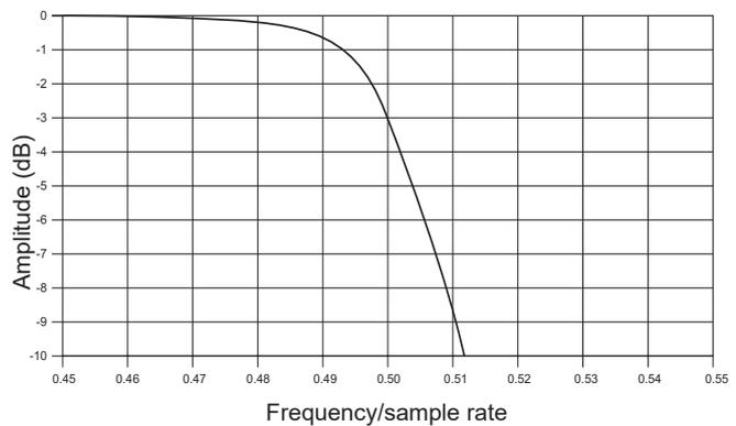
Fig. 8: Sample rate 100 S/s to 51.2 kS/s
