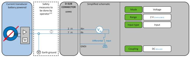
Fig. 51: Current transducer with voltage output
