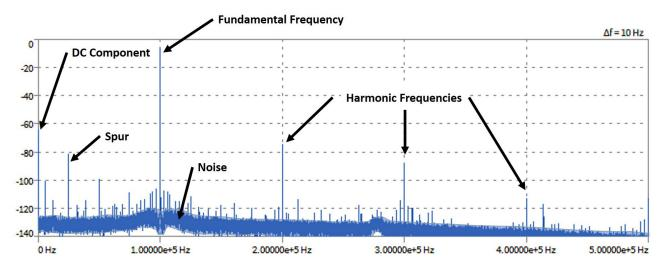
Fig. 221: FFT chart of TRION-1620-ACC
