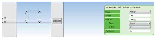
Fig. 27: Voltage measurement
