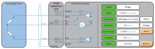
Fig. 60: Half bridge 3-wire
