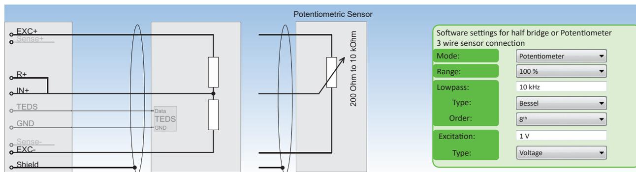
Fig. 64: Half bridge or Potentiometer 3 wire sensor connection
