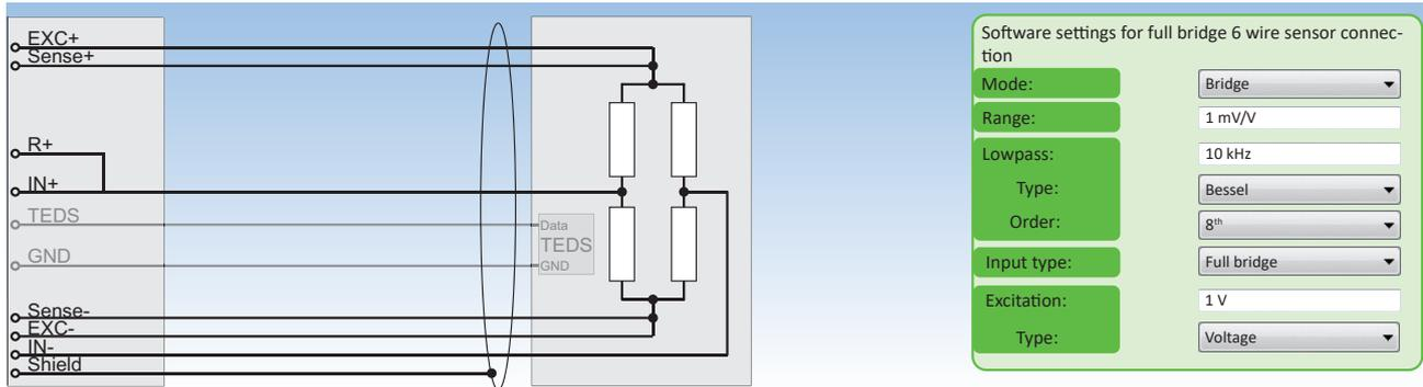
Fig. 61: Full bridge 6-wire sensor connection
