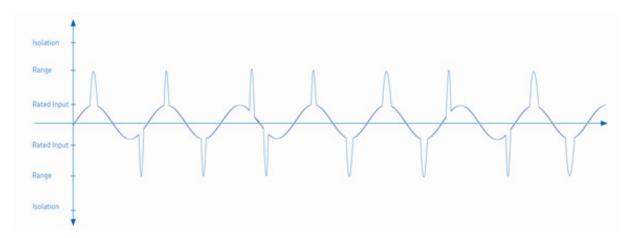
Fig. 215: Relation between rated input, input ranges and isolation voltage
