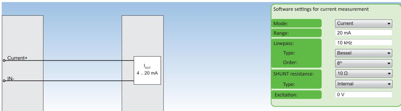
Fig. 95: Current measurement
