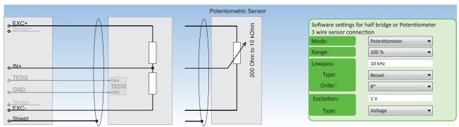
Fig. 83: Half bridge or Potentiometer 3 wire sensor connection
