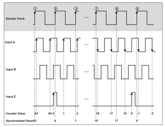
Fig. 201: Quadrature Encoder with channel Z
