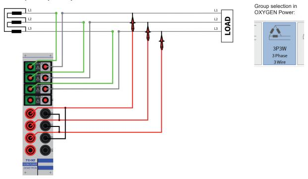
Fig. 144: Three phase (3P3W) without neutral line
