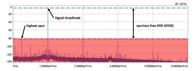
Fig. 222: SFDR in a FFT chart with input signal (alternative method)
