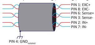
Fig. 91: Cables and shielding
