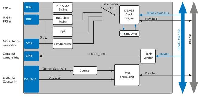
Fig. 170: Signal routing
