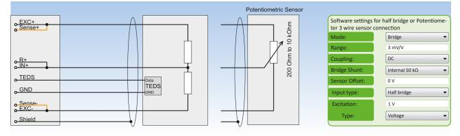
Fig. 111: Half bridge or Potentiometer 3 wire sensor connection
