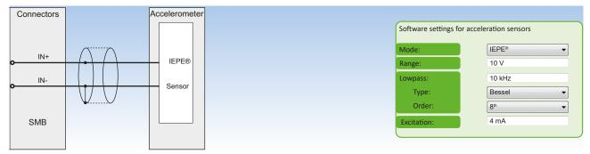
Fig. 32: IEPE<sup>®</sup> sensor (TRION-1620-ACC only)
