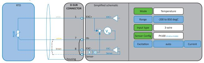
Fig. 67: RTD 3-wire temperature measurement
