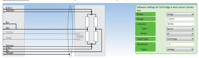
Fig. 81: Full bridge 6-wire sensor connection
