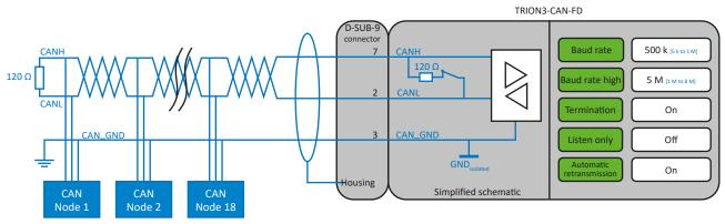
Fig. 206: Connecting sensors via CAN Bus
