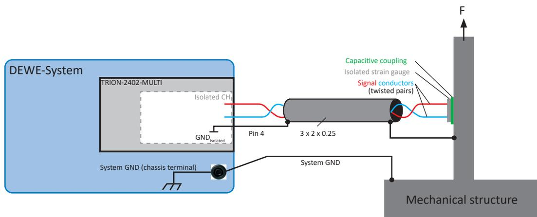
Fig. 73: Strain gauge measurement on a metal structure
