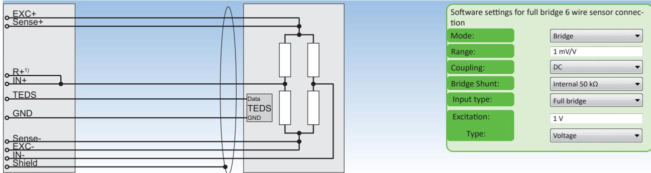
Fig. 121: Full bridge 6-wire sensor connection
