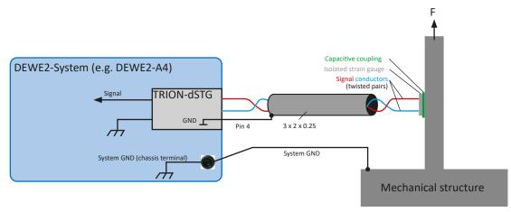
Fig. 118: Strain gauge measurement
