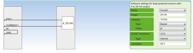
Fig. 31: Loop-powered sensors with 4 to 20 mA output
