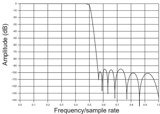
**Input frequency response near the cut-off**
