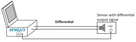
Fig. 124: Sensor with differential output signal
