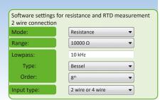
Fig. 87: Resistance and RTD measurement 2 wire connection
