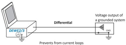
Fig. 124: Voltage output of a grounded system
