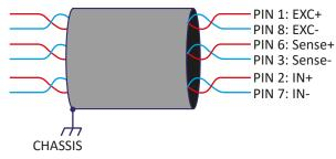
Fig. 74: Cables and shielding
