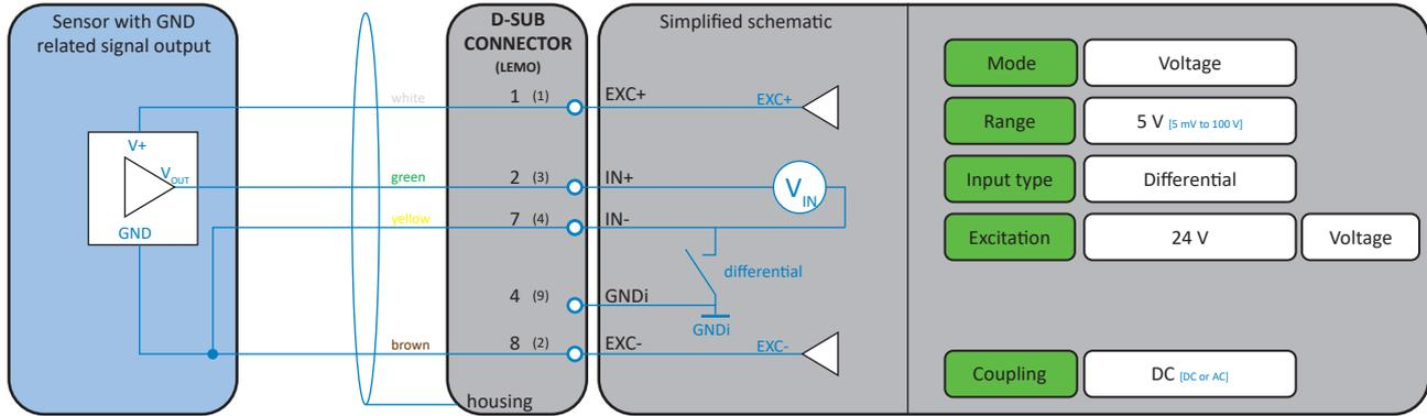
Fig. 30: Single-ended sensor powered by the TRION module
