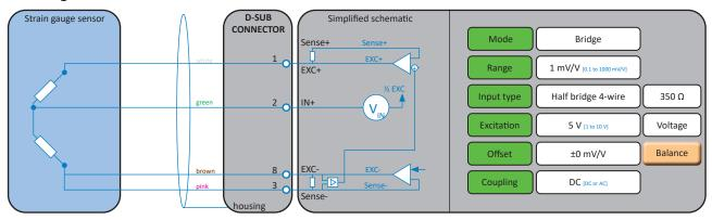
Fig. 58: Half bridge 4-wire
