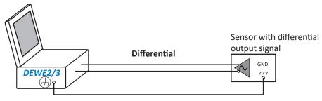
Fig. 123: Sensor with differential output signal
