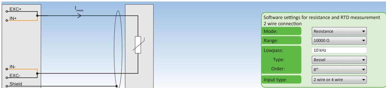
Fig. 67: Resistance and RTD measurement 2 wire connection
