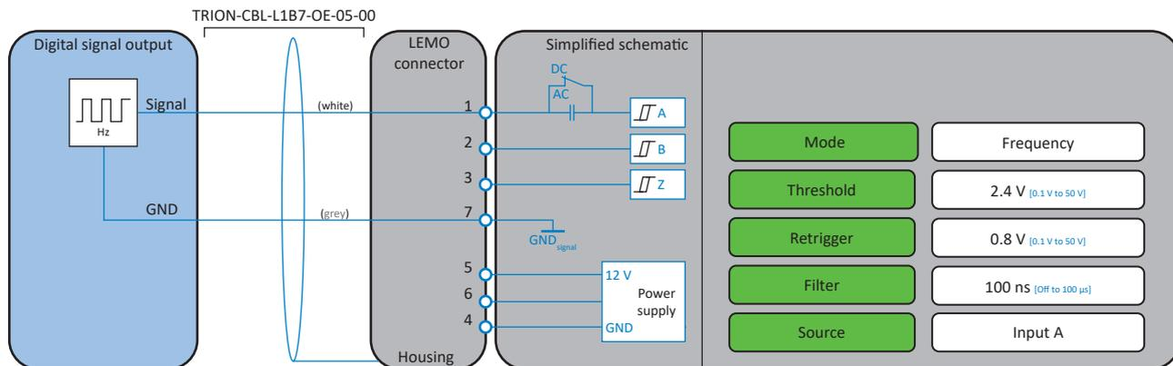
Fig. 195: Frequency (digital output)
