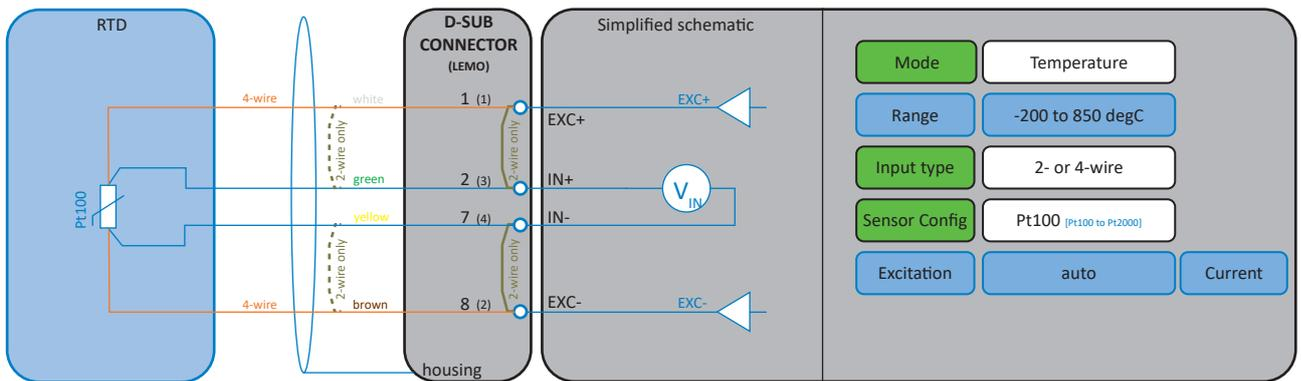
Fig. 47: RTD 2- and 4-wire temperature measurement
