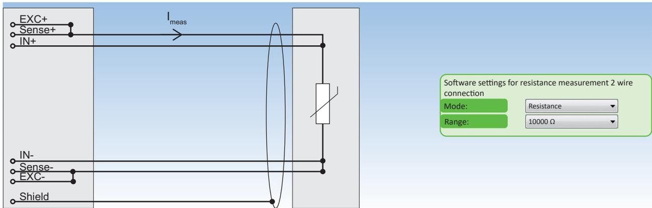
Fig. 128: Resistance and RTD measurement 4 wire connection
