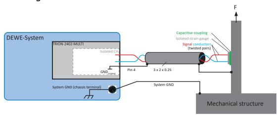
Fig. 93: Strain gauge measurement on a metal structure
