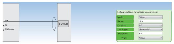
Fig. 104: Voltage measurement
