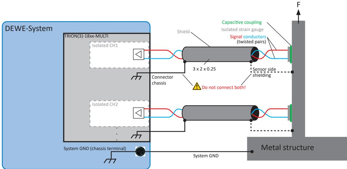
Fig. 55: Strain gauge measurement on a metal structure
