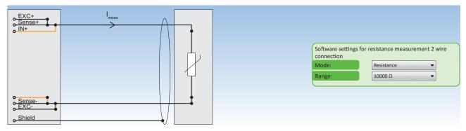
Fig. 113: Resistance and RTD measurement 2 wire connection
