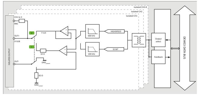
Fig. 164: Analog block diagram
