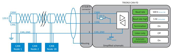
Fig. 206: Connecting sensors via CAN Bus
