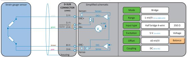
Fig. 59: Half bridge 4-wire
