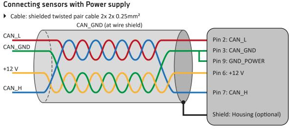
Fig. 211: Cabling for sensors with power supply
