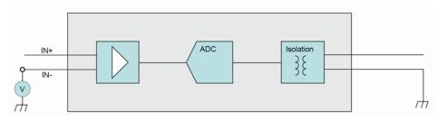
Fig. 229: Isolation voltage
