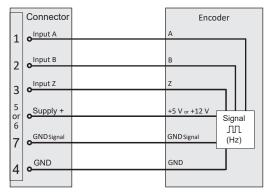
Fig. 167: Supplied sensor connection
