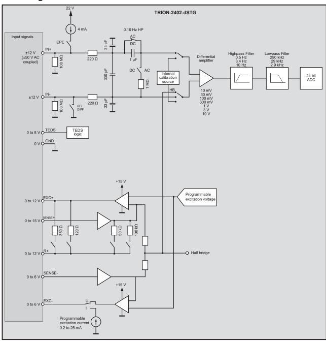
Fig. 118: Block diagram
