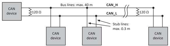
Fig. 212: High-speed CAN
