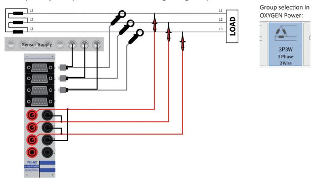
Fig. 146: Three phase (3P3W) without neutral line, using voltage output transducers
