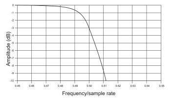
Input frequency response near the cut-off
