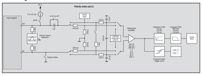
Fig. 119: Block diagram
