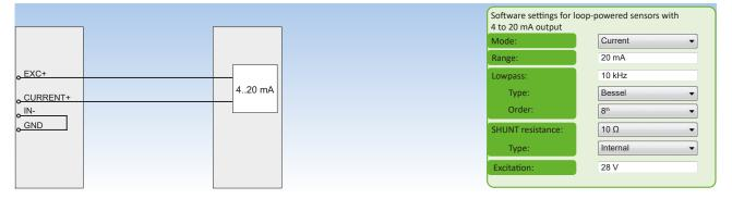
Fig. 41: Loop-powered sensors with 4 to 20 mA output
