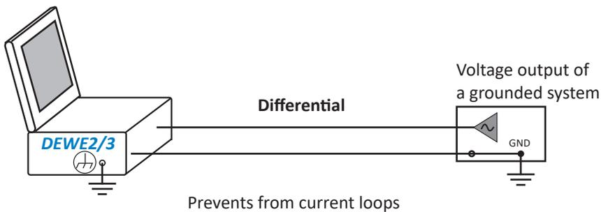
Fig. 138: Voltage output of a grounded system
