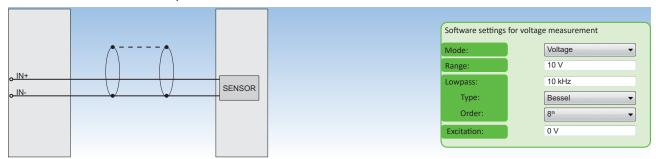
Fig. 27: Voltage measurement
