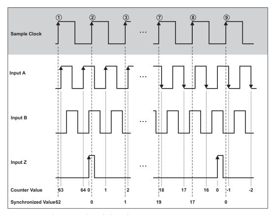
Fig. 194: Quadrature Encoder with channel Z
