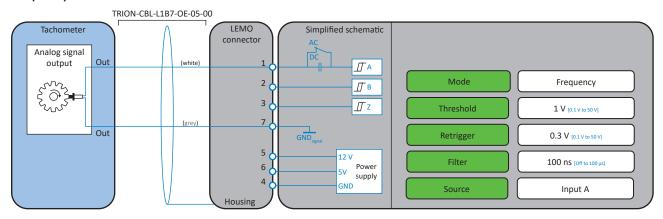
Fig. 185: Frequency measurement (analog output)
