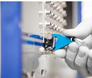
5. Remove the TRION(3) module and reinstall the filler panel into the empty slot.
