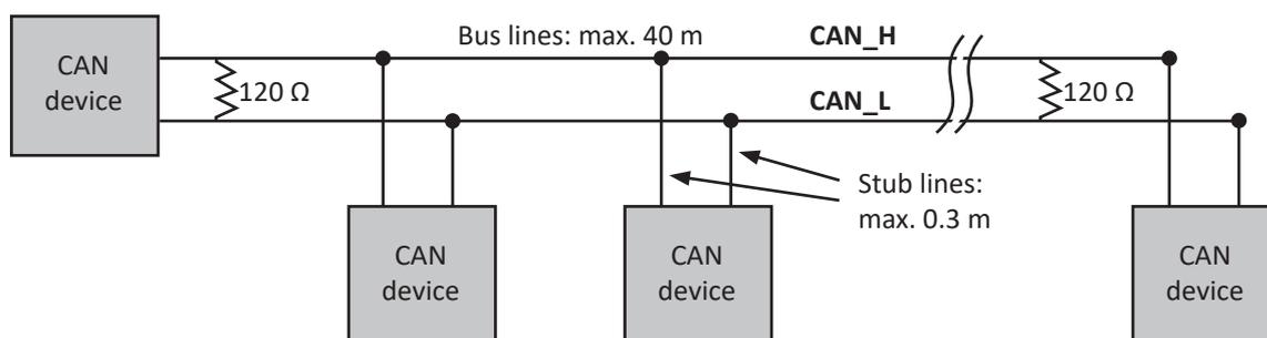
Fig. 225: High-speed CAN
