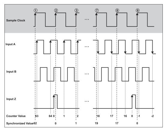
Fig. 201: Quadrature Encoder with channel Z
