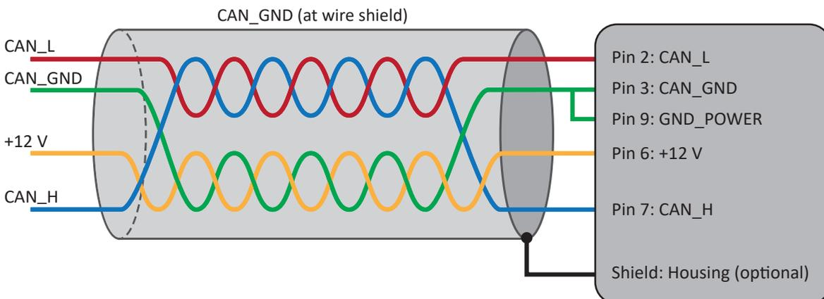
Fig. 224: Cabling for sensors with power supply
