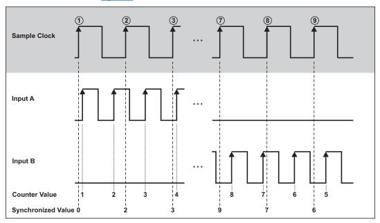
Fig. 195: A-Up/B-down encoder
