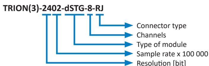
Fig. 1: Decoding a TRION(3) series module
