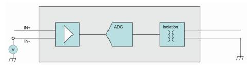
Fig. 213: Isolation voltage
