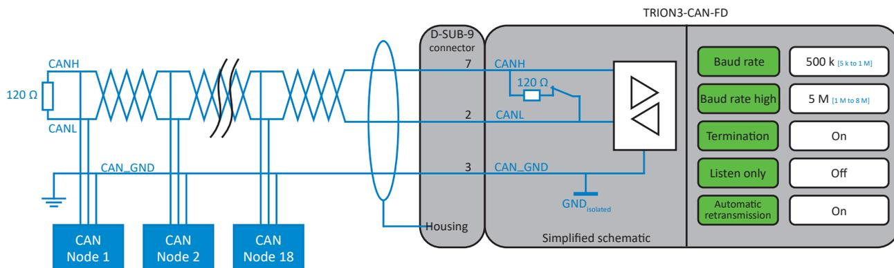
Fig. 219: Connecting sensors via CAN Bus
