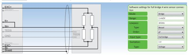
Fig. 82: Full bridge 4-wire sensor connection
