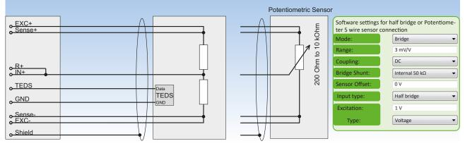
Fig. 110: Half bridge or Potentiometer 5 wire sensor connection
