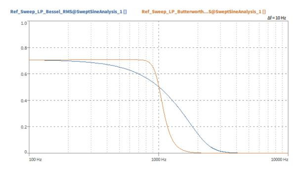
Fig. 141: Frequency response of filter with 1000 Hz cutoff frequency and 8th order
