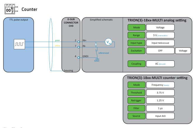
Fig. 68: Counter measurement
