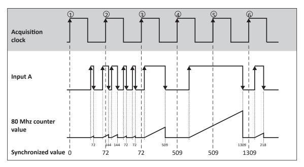
Fig. 196: Pulse width measurement
