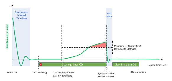
Fig. 175: Forced restart after restored synchronization
