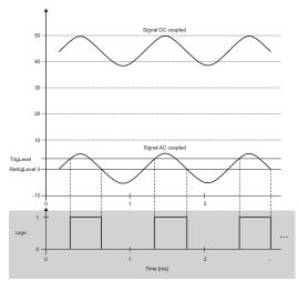
Fig. 191: Programmable trigger level
