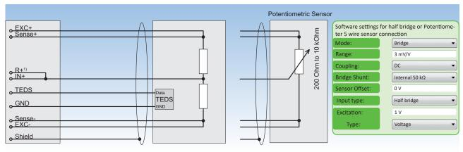
Fig. 109: Half bridge or Potentiometer 5 wire sensor connection
