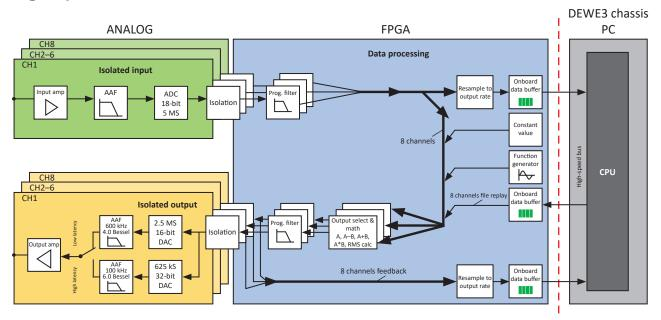
Fig. 45: Simplified signal path
