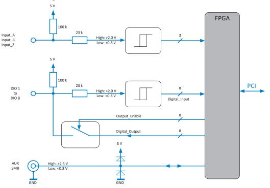
Fig. 172: Counter and digital I/O
