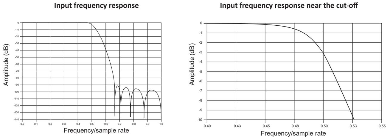
Fig. 9: Sample rate 51.2 kS/s to 102.4 kS/s
