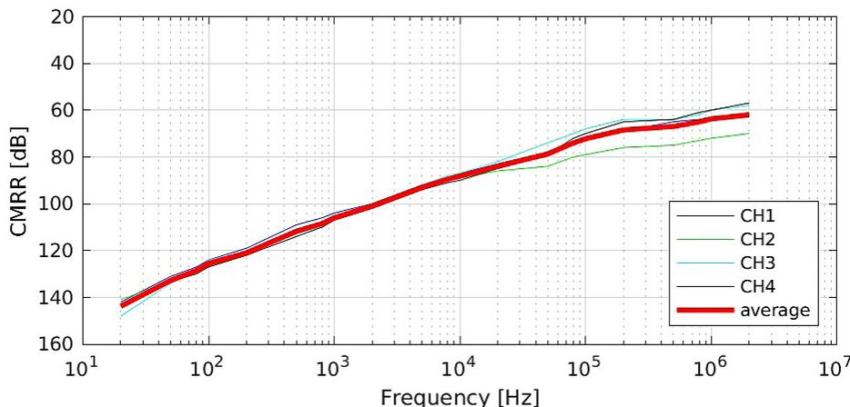
Fig. 241: CMRR over frequency response of a TRION-1820-POWER-4 (V inputs) (not a directly measured FFT chart)
