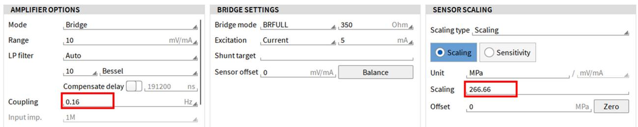
Fig. 45: Scaling settings in OXYGEN
