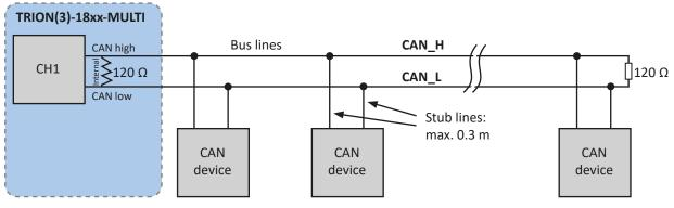
Fig. 73: CAN bus connection
