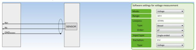
Fig. 78: Voltage measurement
