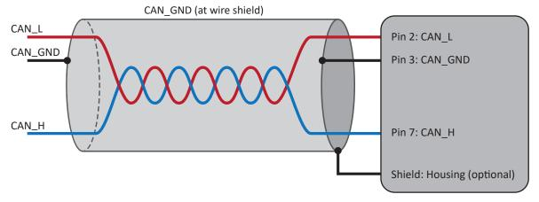
Fig. 209: Cabling for light industrial environment
