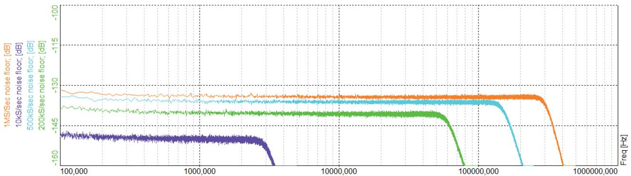
Fig. 15: Noise floor of TRION-1620-ACC at different sample rates
