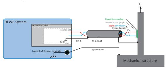
Fig. 92: Strain gauge measurement on a metal structure
