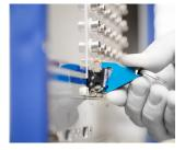
5. Remove the TRION(3) module and reinstall the filler panel into the empty slot.
