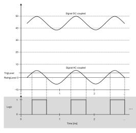
Fig. 191: Programmable trigger level
