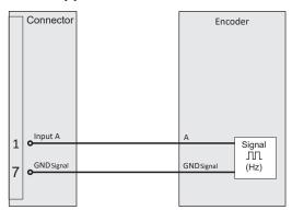
Fig. 167: Non-supplied sensor connection
