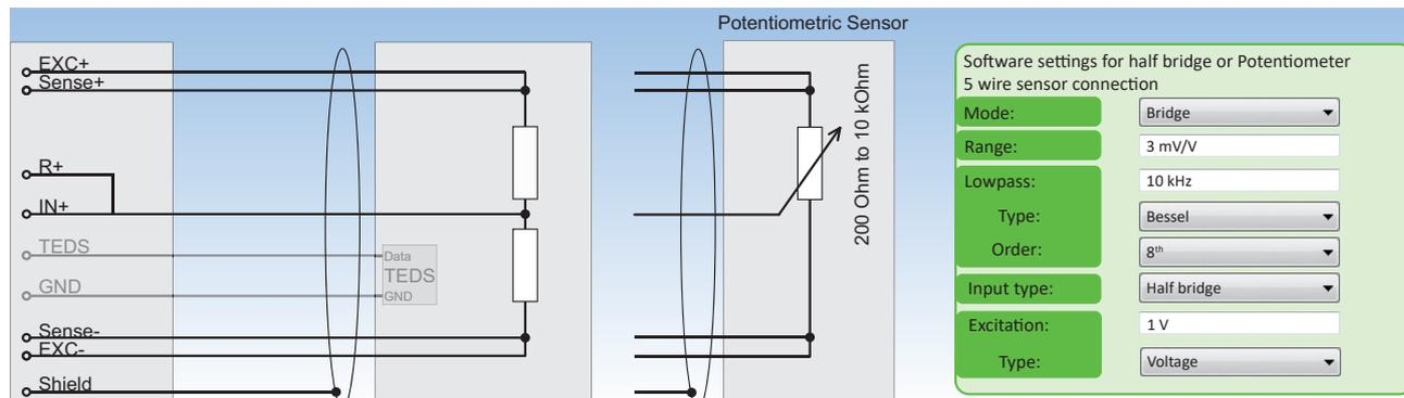
Fig. 63: Half bridge or Potentiometer 5 wire sensor connection
