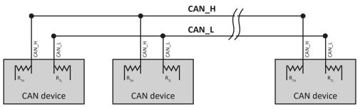
Fig. 213: Low-speed / fault-tolerant CAN
