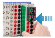
**8.** Pull up the injector/ejector handle to latch the module. Tighten the screws at the top and bottom of the TRION(3) module front panel (4x) to secure the module.
