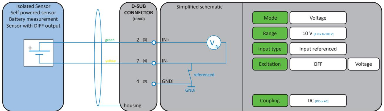
Fig. 28: Voltage measurement
