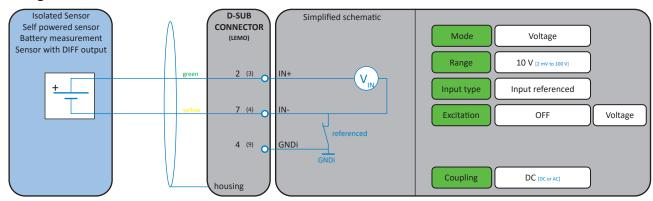
Fig. 48: Voltage measurement
