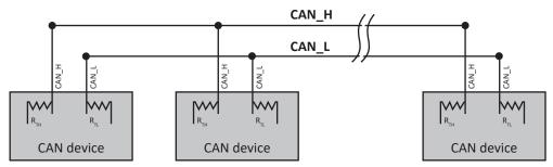
Fig. 199: Low-speed / fault-tolerant CAN
