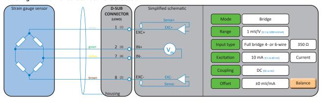
Fig. 57: Full bridge 4-wire with constant current excitation
