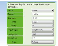
Fig. 85: Quarter bridge 3 wire sensor connection
