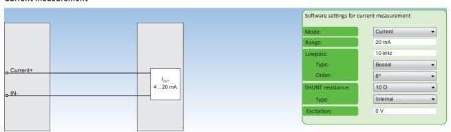
Fig. 29: Current measurement
