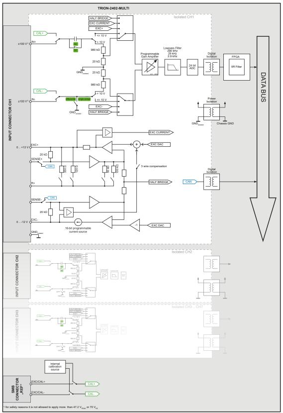
Fig. 94: Block diagram
