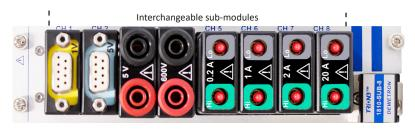
*Fig. 156: Connection ports*
