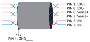
Fig. 92: Cables and shielding
