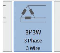
Fig. 157: Three phase (3P3W) without neutral line
