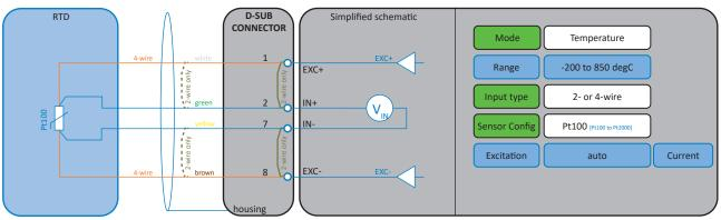
Fig. 66: RTD 2- and 4-wire temperature measurement
