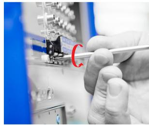
4. Pull down the injector/ejector handle or use the TRION extraction tool to release the module.
