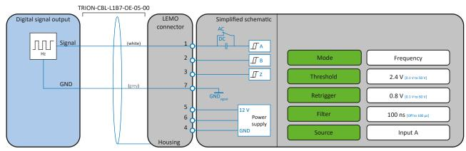
Fig. 182: Frequency (digital output)
