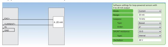
Fig. 41: Loop-powered sensors with 4 to 20 mA output
