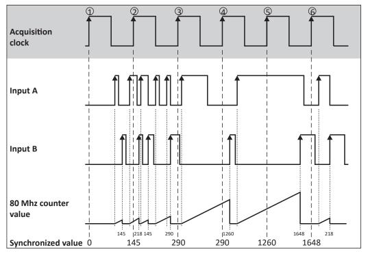
Fig. 190: Two Pulse Edge Separation Measurement
