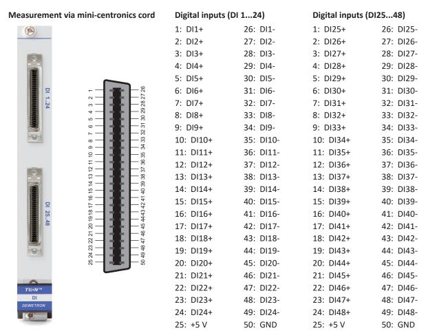
Fig. 202: 50-pin mini-centronics socket
