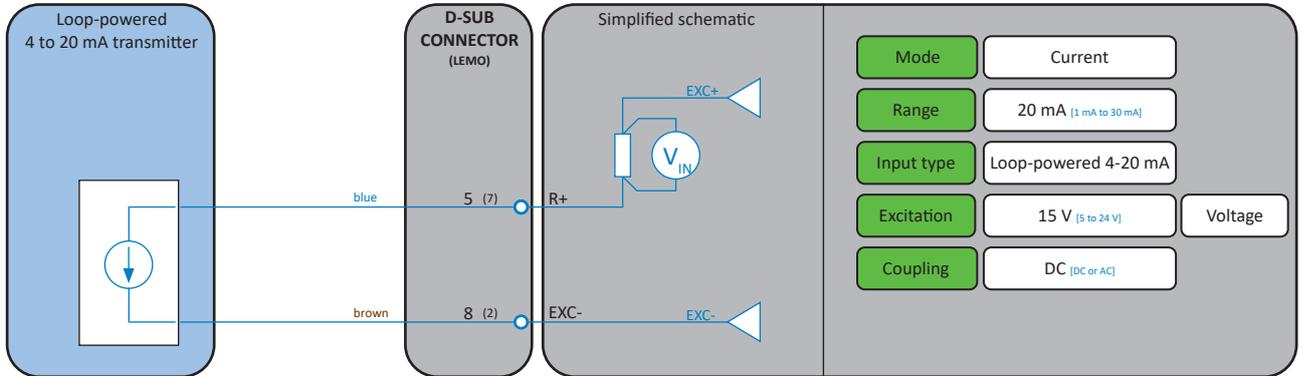
Fig. 32: Loop-powered 4 to 20 mA transmitter
