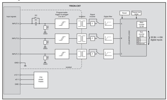
Fig. 190: Block diagram
