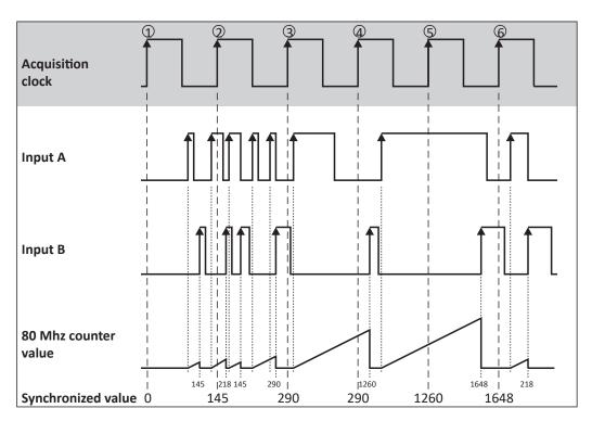
Fig. 197: Two Pulse Edge Separation Measurement
