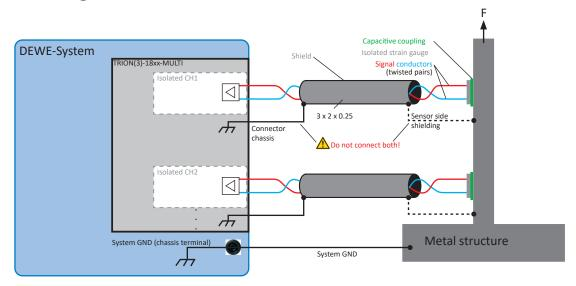
Fig. 75: Strain gauge measurement on a metal structure
