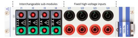
Fig. 135: Connection ports
