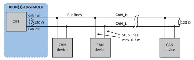
Fig. 72: CAN bus connection
