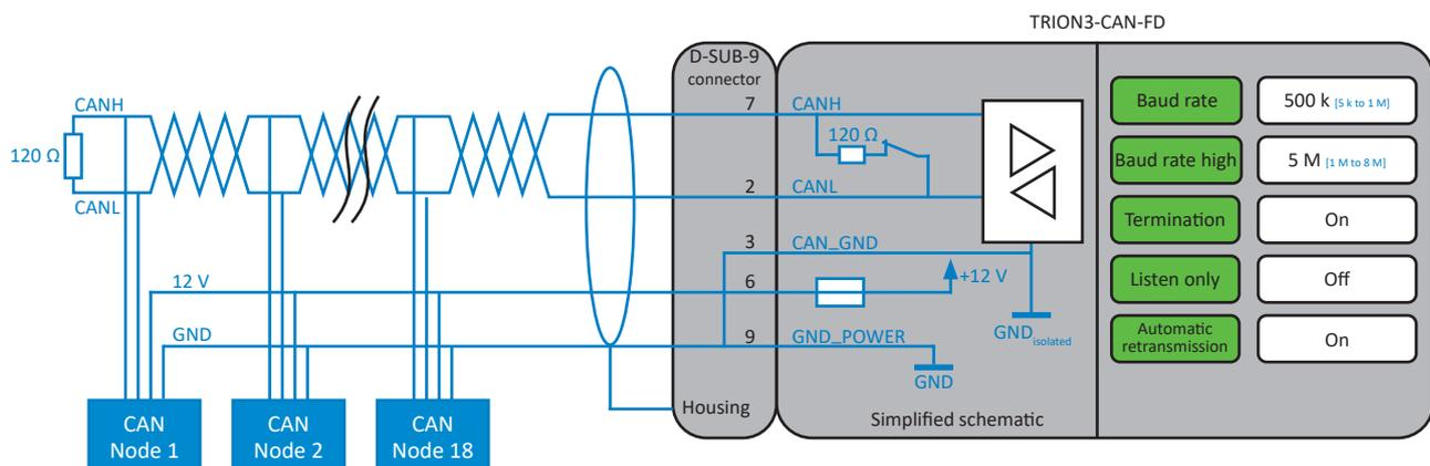
Fig. 220: Connecting sensors directly supplied by TRION3-CAN-FD
