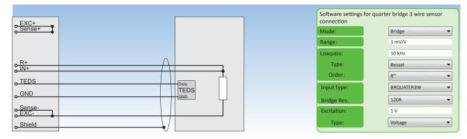
Fig. 84: Quarter bridge 3 wire sensor connection
