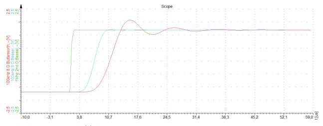
Fig. 12: Step response TRION(3)-18xx-MULTI series
