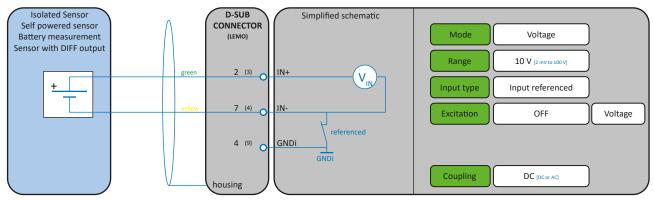
Fig. 48: Voltage measurement
