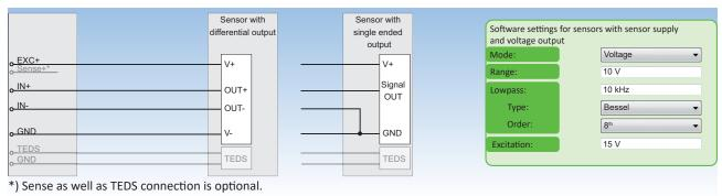
Fig. 28: Sensors with sensor supply and voltage output
