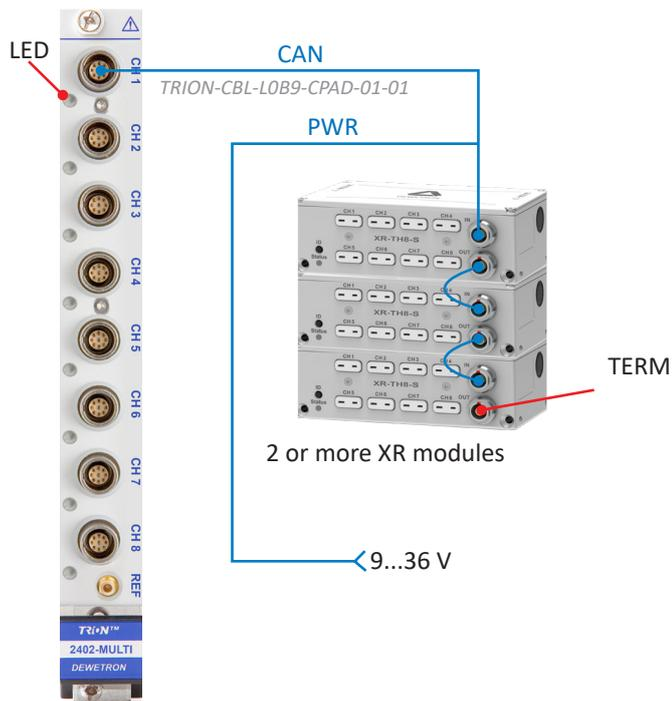
Fig. 71: Connecting XR modules to the TRION-2402-MULTI module
