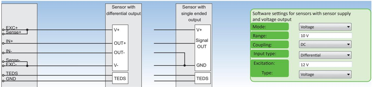
Fig. 119: Sensors with sensor supply and voltage output
