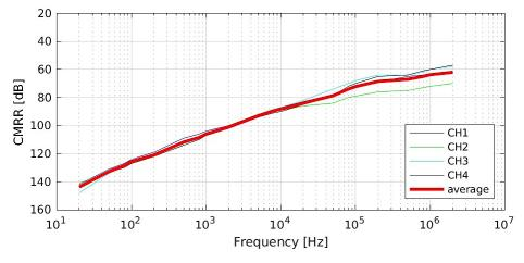
Fig. 212: CMRR over frequency response of a TRION-1820-POWER-4 (V inputs) (not a directly measured FFT chart)
