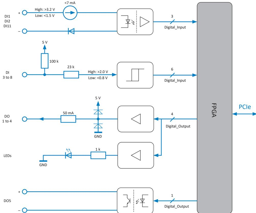
Fig. 82: Digital block diagram
