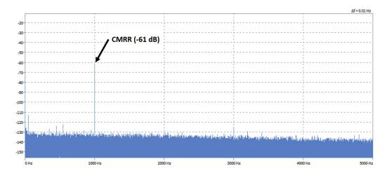
Fig. 227: Measurement of CMRR in FFT chart of TRION-1620-ACC (>2 V range @ 1 kHz)
