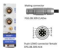
1: EXC+ (CAN power supply 12 V, CH1 only) 2: EXC-3: IN+ 4: IN-5: SENSE+ (CAN high, CH1 only) 6: SENSE- (CAN low, CH1 only) 7: R+ 8: TEDS 9: GND<sub>isolated</sub> (CAN GND, CH1 only) Housing connected to chassis GND
