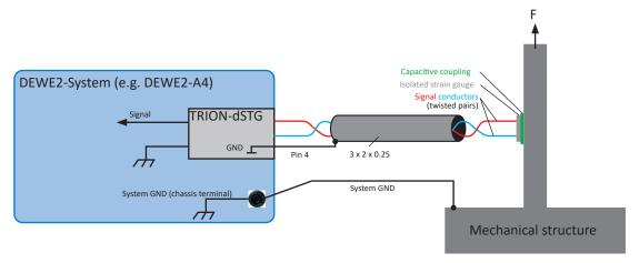
Fig. 118: Strain gauge measurement
