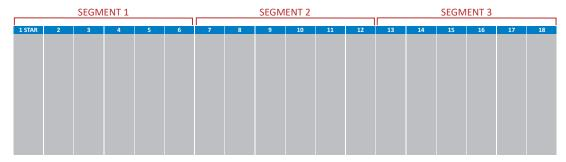
Fig. 6: Slots for DEWE2-M13/M13s/M18 devices
