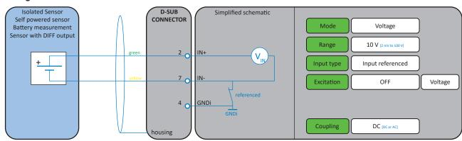
Fig. 48: Voltage measurement
