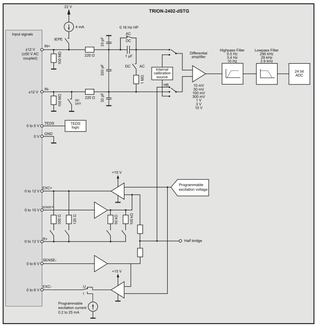
Fig. 119: Block diagram
