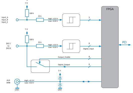
Fig. 171: Counter and digital I/O
