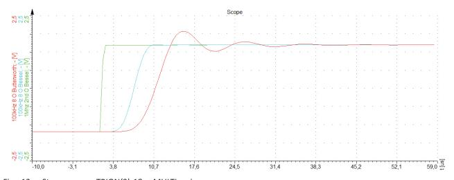
Fig. 12: Step response TRION(3)-18xx-MULTI series
