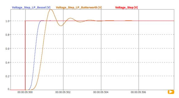
Fig. 141: Step response of filter with 1000 Hz cutoff frequency and 8th order.
