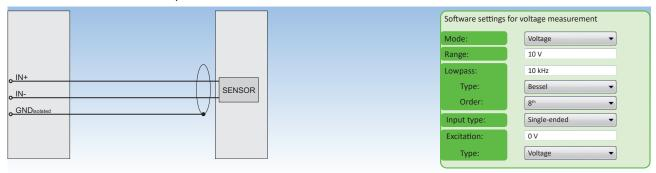
Fig. 77: Voltage measurement
