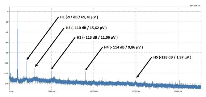
Fig. 225: THD measurement of TRION-1802/1600-dLV-32 (@50 kS/s) where Uf = 4.94 V equals 0 dB
