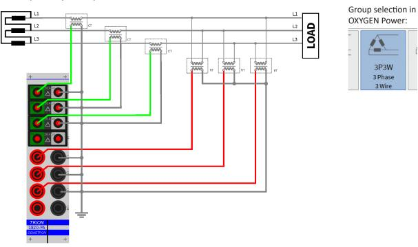
Fig. 147: Three phase (3P3W) with CT and VT
