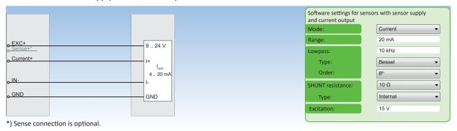
Fig. 30: Sensors with sensor supply and current output
