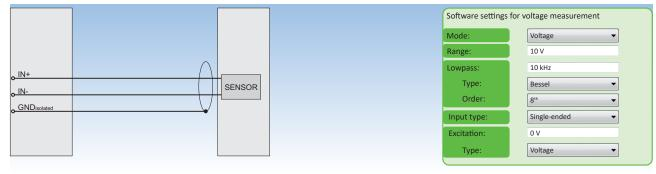
Fig. 78: Voltage measurement
