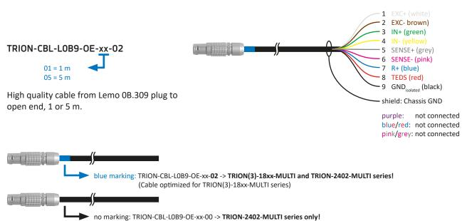
INFORMATION Using the pre-configured LEMO connector with cable is highly recommended because manually soldering the OB LEMO connector is tricky. The wire colors are also mentioned in the signal connection section to amplify sensor connection.
