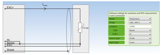
Fig. 88: Resistance and RTD measurement 3 wire connection
