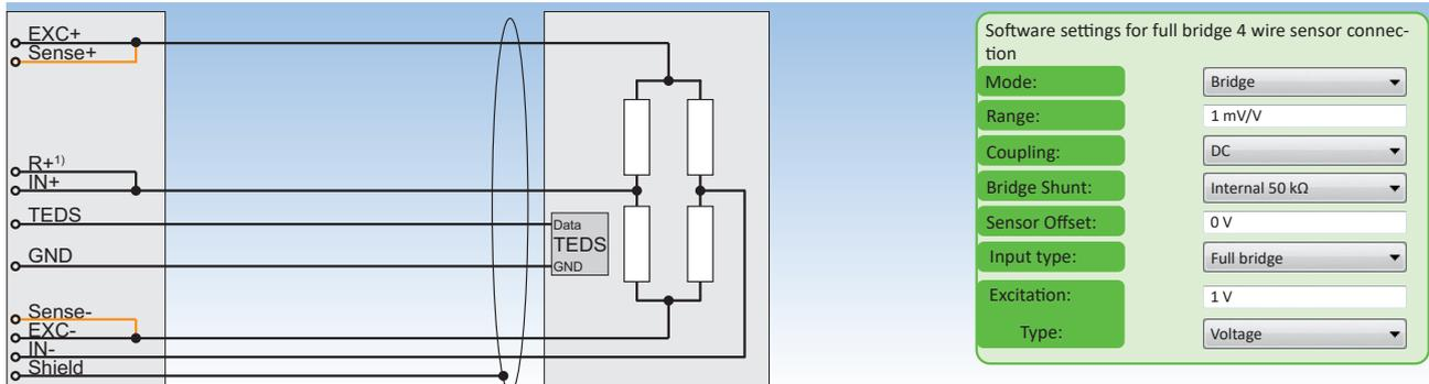
Fig. 122: Full bridge 4-wire sensor connection
