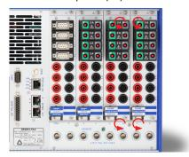
The TRION sub-module is now exchanged.
