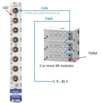
Fig. 76: Connecting XR modules to the TRION(3)-18xx-MULTI
