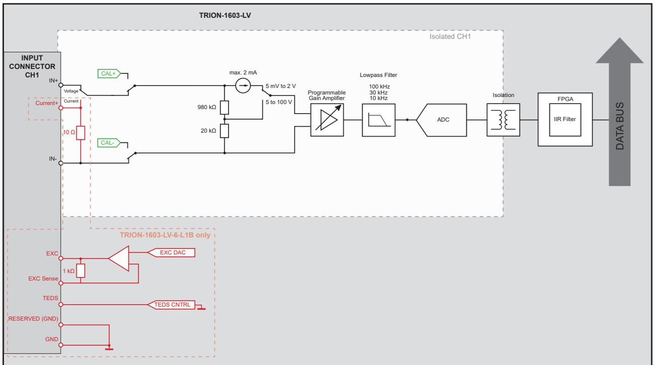
Fig. 102: Base block diagram of the TRION-1603-LV module
