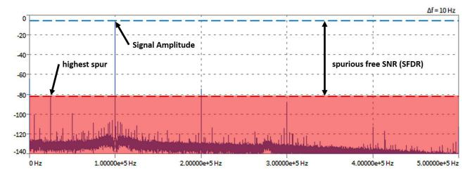
Fig. 222: SFDR in a FFT chart with input signal (alternative method)
