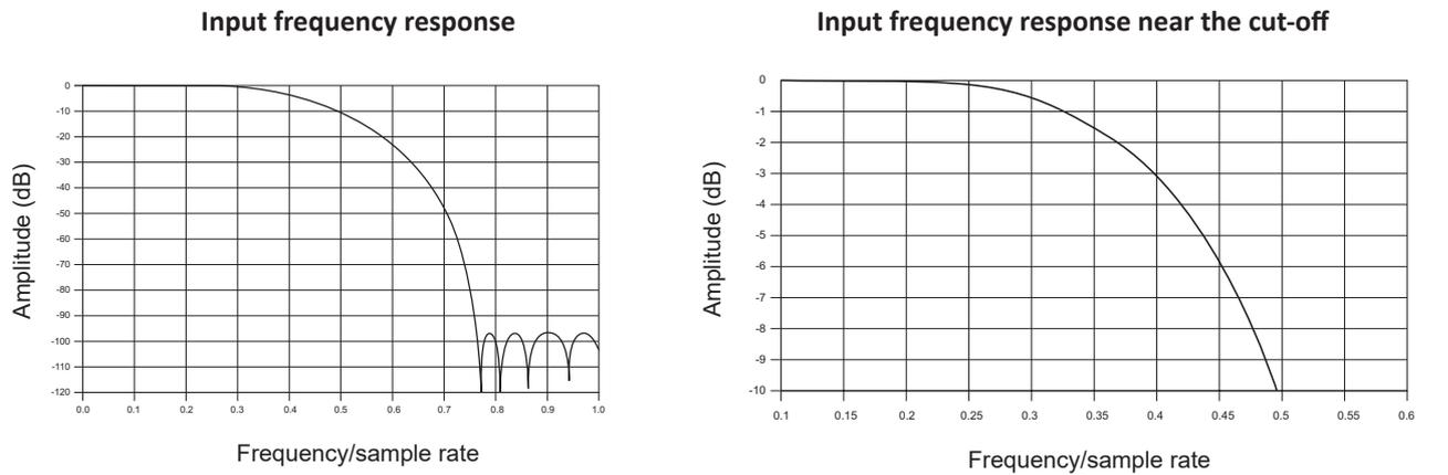
Fig. 10: Sample rate 102.4 kS/s to 200 kS/s
