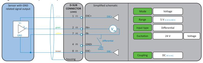
Fig. 50: Single-ended sensor powered by the TRION module
