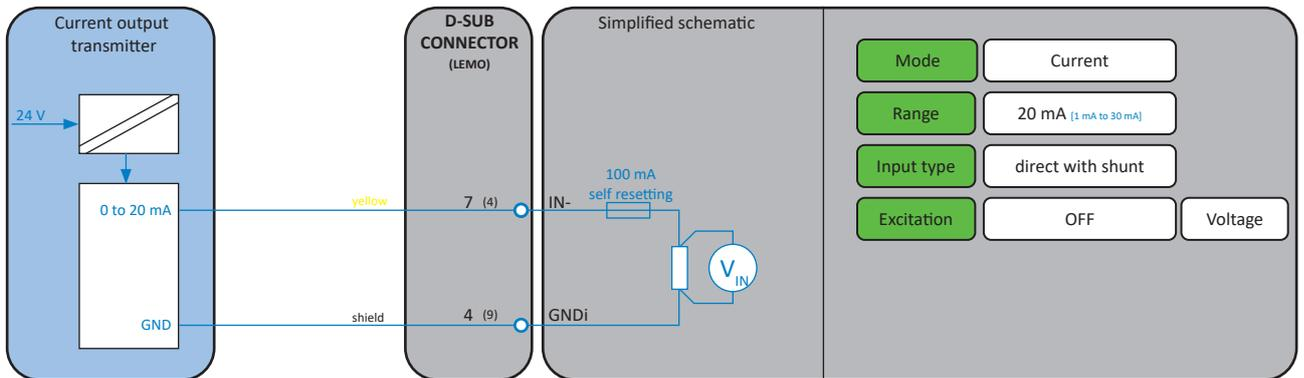
Fig. 33: Current measurement (with externally powered transmitter)
