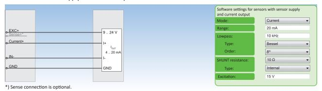
Fig. 40: Sensors with sensor supply and current output
