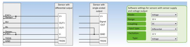
Fig. 106: Sensors with sensor supply and voltage output
