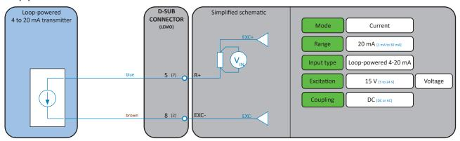
Fig. 52: Loop-powered 4 to 20 mA transmitter
