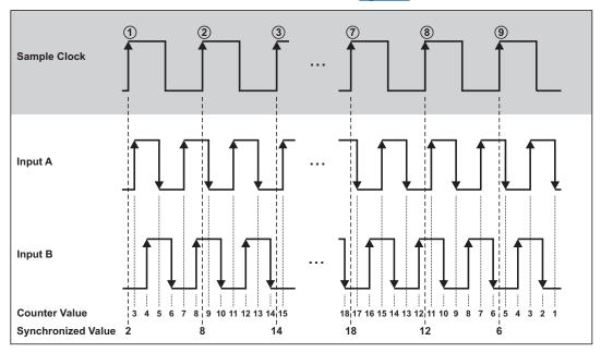
Fig. 200: Quadrature Encoder X4 Mode
