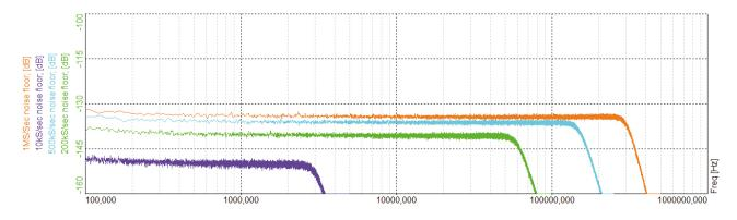
Fig. 15: Noise floor of TRION-1620-ACC at different sample rates
