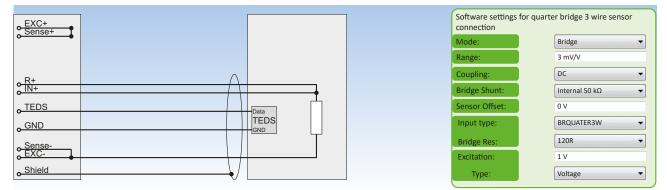
Fig. 112: Quarter bridge 3 wire sensor connection
