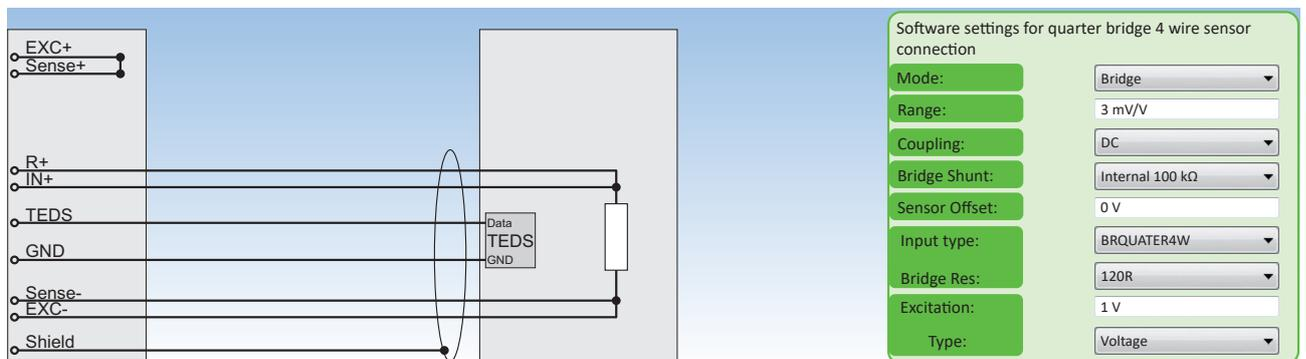
Fig. 126: Quarter bridge 4 wire sensor connection
