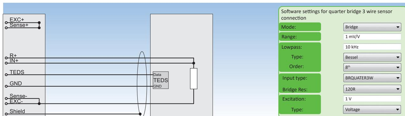
Fig. 65: Quarter bridge 3 wire sensor connection
