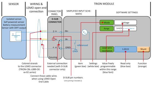
Fig. 47: Reading schematics
