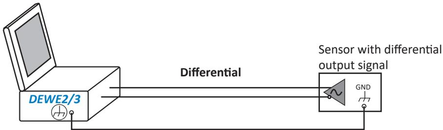
Fig. 137: Sensor with differential output signal
