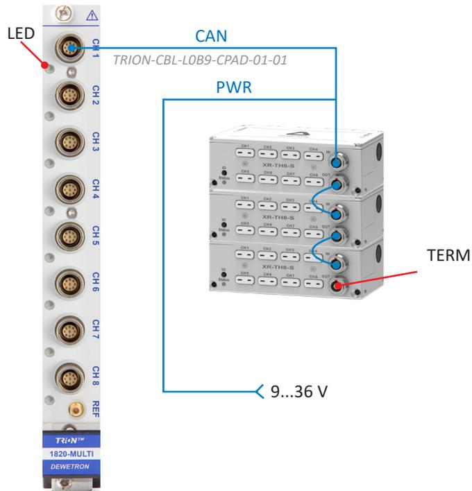
Fig. 56: Connecting XR modules to the TRION(3)-18xx-MULTI
