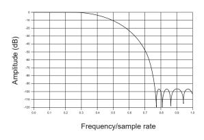
Input frequency response near the cut-off
