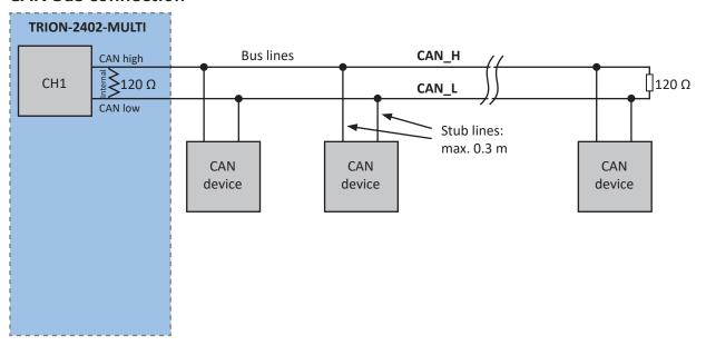
Fig. 89: CAN bus connection
