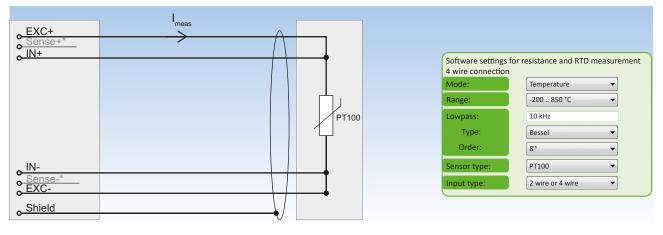
Fig. 89: Resistance and RTD measurement 4 wire connection
