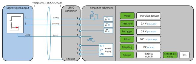
Fig. 183: Two pulse edge separation
