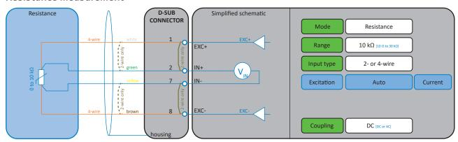
Fig. 65: Resistance measurement
