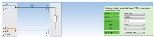
Fig. 87: Resistance and RTD measurement 2 wire connection
