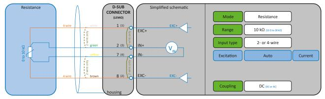
Fig. 66: Resistance measurement
