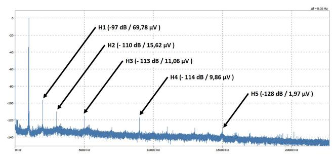
Fig. 225: THD measurement of TRION-1802/1600-dLV-32 (@50 kS/s) where Uf = 4.94 V equals 0 dB Formula
