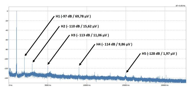
Fig. 209: THD measurement of TRION-1802/1600-dLV-32 (@50 kS/s) where Uf = 4.94 V equals 0 dB
