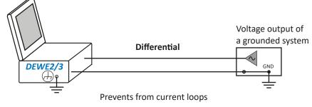
Fig. 125: Voltage output of a grounded system
