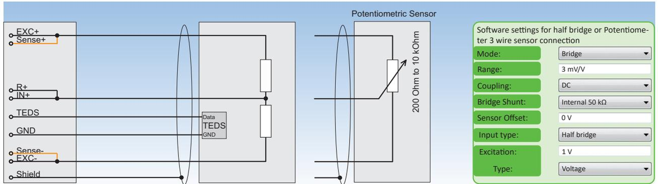
Fig. 124: Half bridge or Potentiometer 3 wire sensor connection
