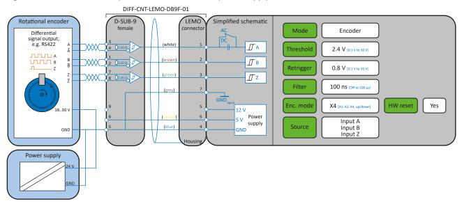
Fig. 188: Rotational encoder externally powered
