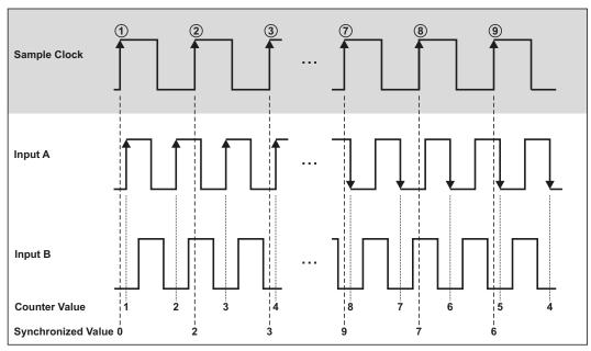
Fig. 198 shows the resulting increments and decrements for X1 encoding.
