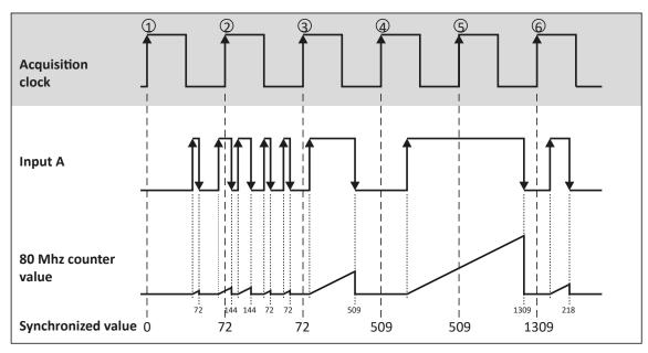
*Fig. 196: Pulse width measurement*
