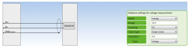
Fig. 105: Voltage measurement
