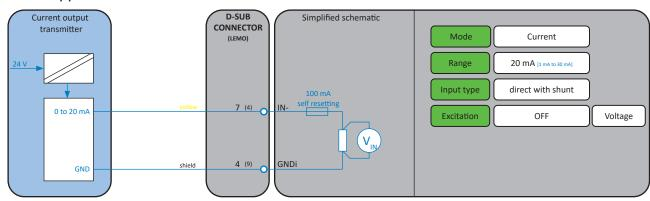
Fig. 53: Current measurement (with externally powered transmitter)
