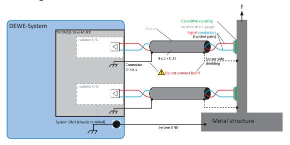
Fig. 74: Strain gauge measurement on a metal structure
