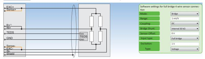
Fig. 109: Full bridge 4-wire sensor connection
