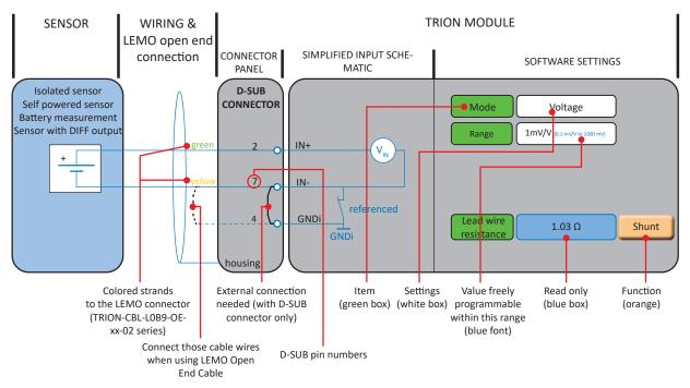
Fig. 47: Reading schematics
