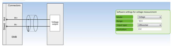
Fig. 126: Voltage measurement
