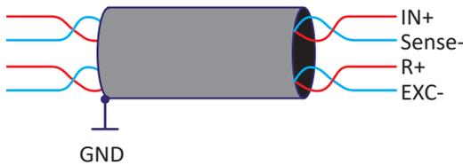
Fig. 130: Cables and shielding for full bridge, half bridge and voltage modes
