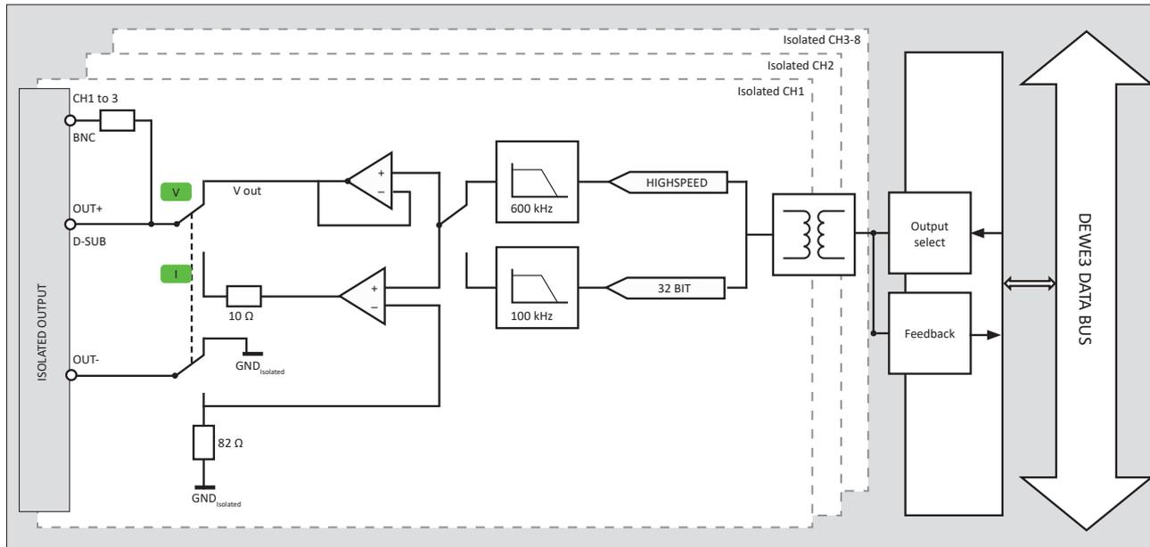
Fig. 177: Analog block diagram
