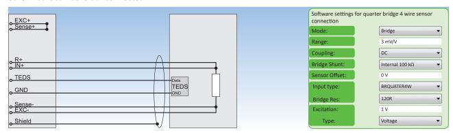
Fig. 113: Quarter bridge 4 wire sensor connection
