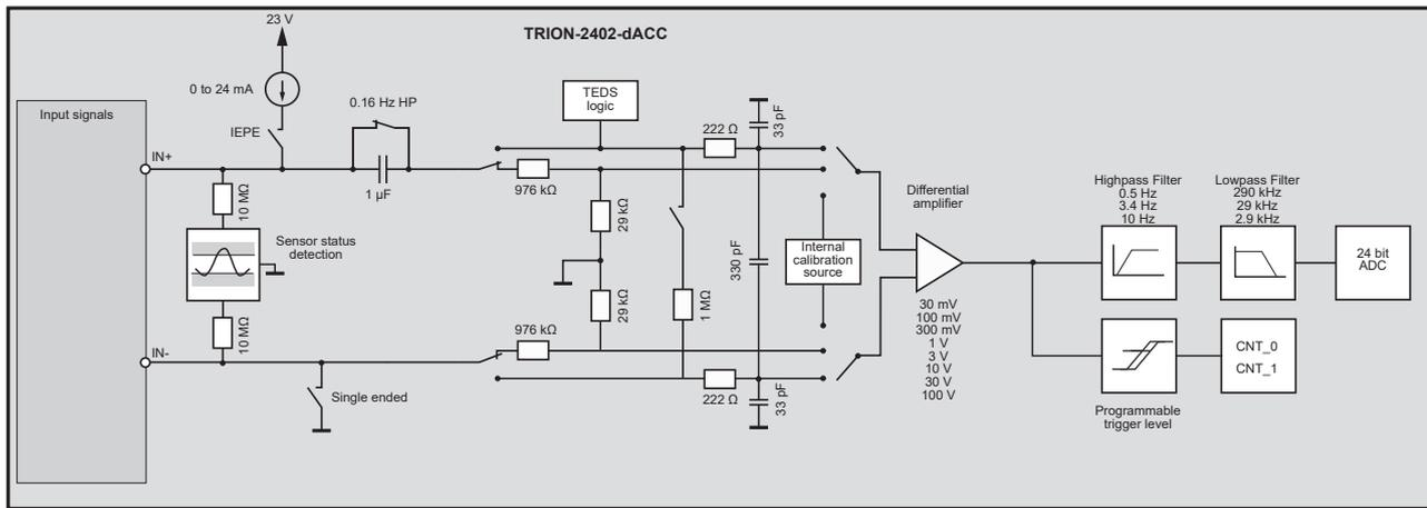
Fig. 133: Block diagram
