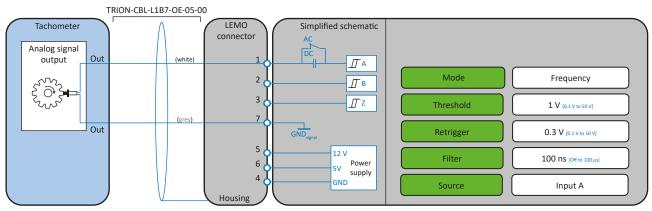
Fig. 185: Frequency measurement (analog output)
