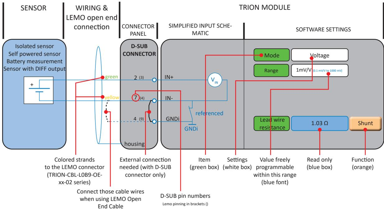
Fig. 27: Reading schematics
