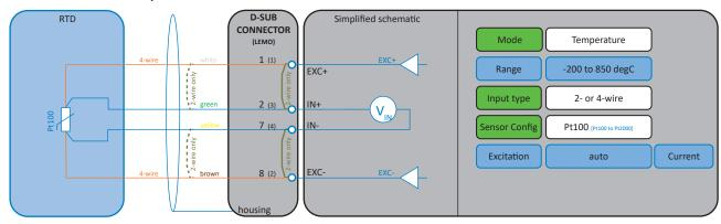
Fig. 67: RTD 2- and 4-wire temperature measurement
