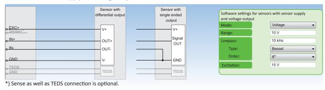
Fig. 38: Sensors with sensor supply and voltage output
