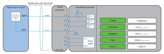
Fig. 182: Frequency (digital output)
