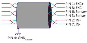
Fig. 92: Cables and shielding
