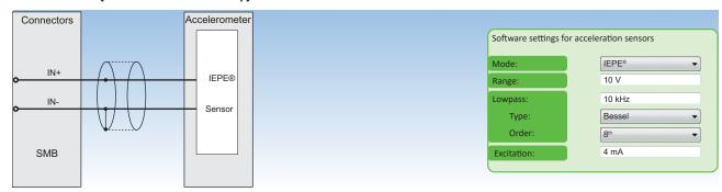
Fig. 32: IEPE® sensor (TRION-1620-ACC only)
