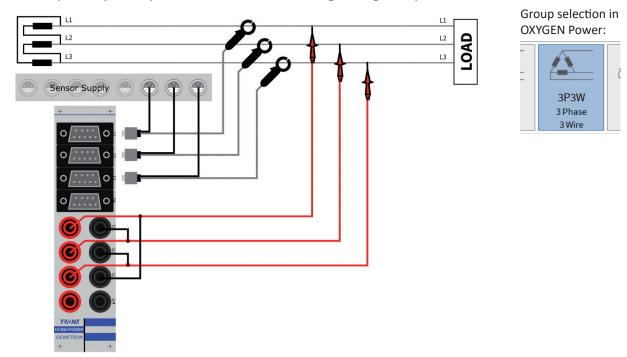
Fig. 145: Three phase (3P3W) without neutral line, using voltage output transducers
