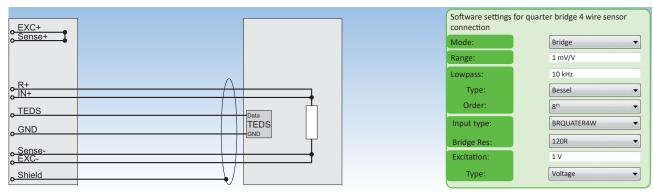
Fig. 85: Quarter bridge 4 wire sensor connection
