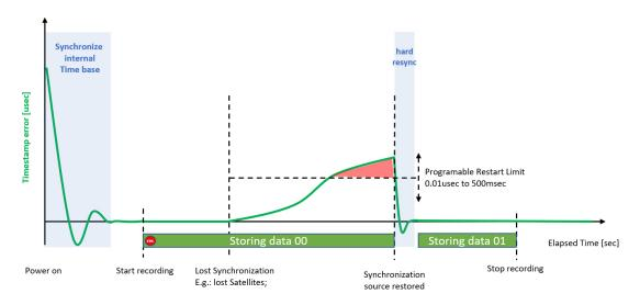
Fig. 174: Forced restart after restored synchronization
