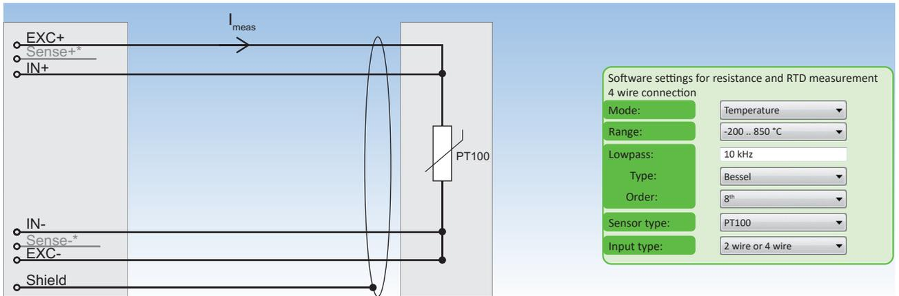
Fig. 69: Resistance and RTD measurement 4 wire connection
