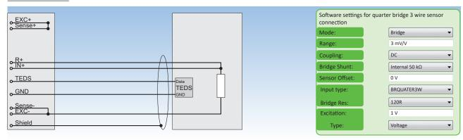
Fig. 111: Quarter bridge 3 wire sensor connection
