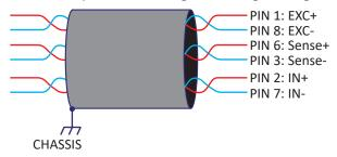
Fig. 74: Cables and shielding
