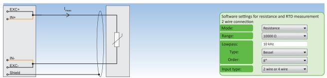
Fig. 86: Resistance and RTD measurement 2 wire connection
