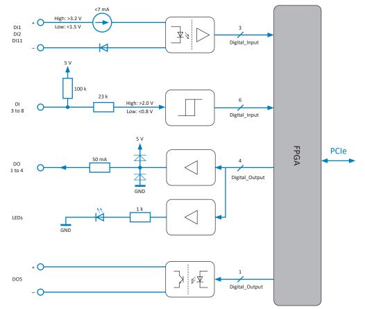
Fig. 164: Digital block diagram
