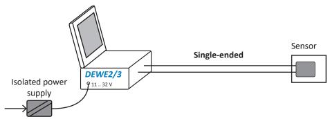
Fig. 121: Isolated power supply/sensor
