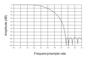
Input frequency response near the cut-off
