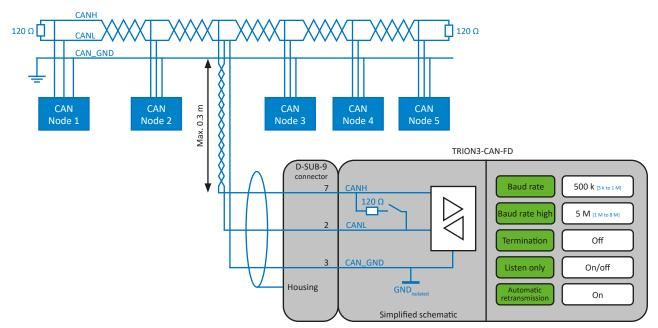
Fig. 205: Analyzing or monitoring a CAN bus
