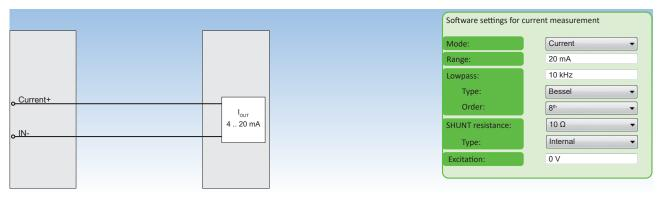
Fig. 29: Current measurement
