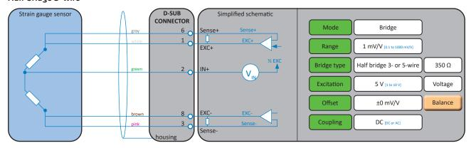
Fig. 57: Half bridge 5-wire
