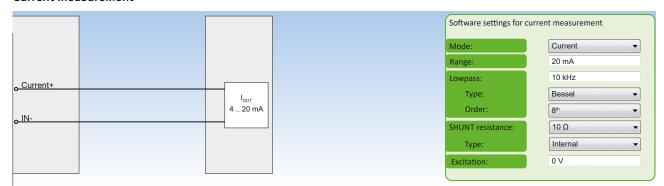
Fig. 39: Current measurement
