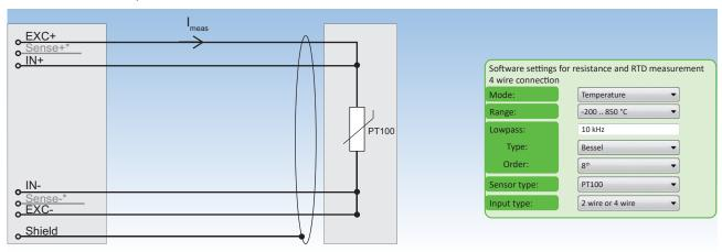
Fig. 88: Resistance and RTD measurement 4 wire connection
