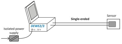
Fig. 122: Isolated power supply/sensor
