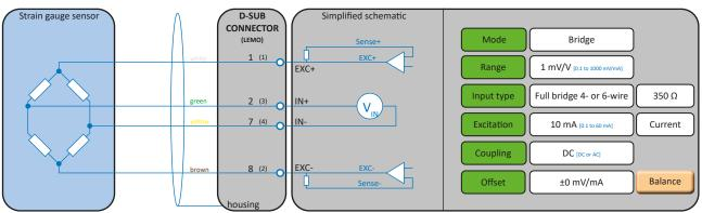
Fig. 57: Full bridge 4-wire with constant current excitation
