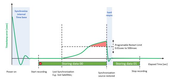
Fig. 175: Forced restart after restored synchronization
