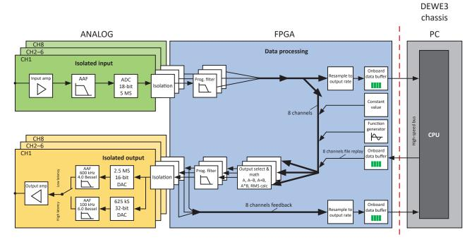
Fig. 45: Simplified signal path
