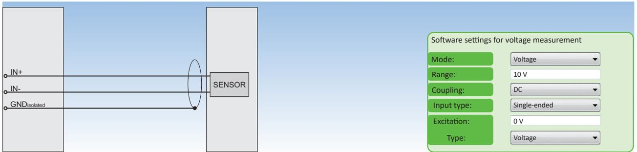
Fig. 118: Voltage measurement
