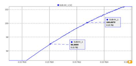
Fig. 219: TRION-SUB-XV auto ranging 100 V  $\leftrightarrow$  1000 V switch over
