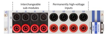
Fig. 128: Connection ports
