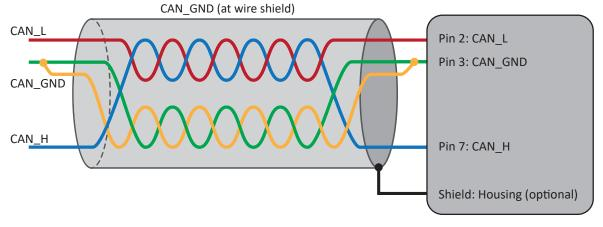
Fig. 210: Cabling for heavy industrial environment
