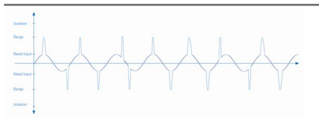
Fig. 231: Relation between rated input, input ranges and isolation voltage
