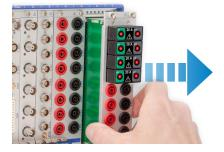
**4.** Loosen the torx screw (M2x4, TX6) which secures the sub-module of the channel you want to replace.
