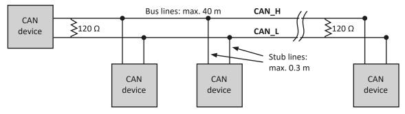
Fig. 212: High-speed CAN
