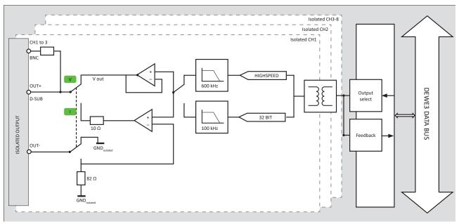
Fig. 164: Analog block diagram
