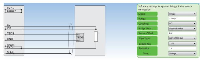
Fig. 112: Quarter bridge 3 wire sensor connection
