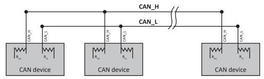
Fig. 213: Low-speed / fault-tolerant CAN
