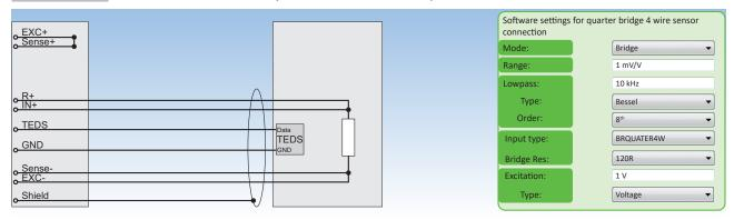
Fig. 86: Quarter bridge 4 wire sensor connection
