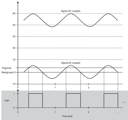
Fig. 204: Programmable trigger level
