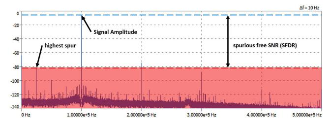
Fig. 206: SFDR in a FFT chart with input signal (alternative method)
