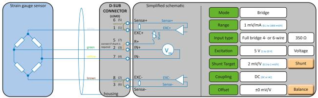
\*) Optional: might be installed on existing sensor cables from previous amplifier series.
