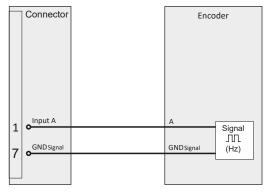
Fig. 168: Non-supplied sensor connection
