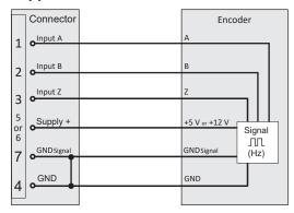
Fig. 180: Supplied sensor connection
