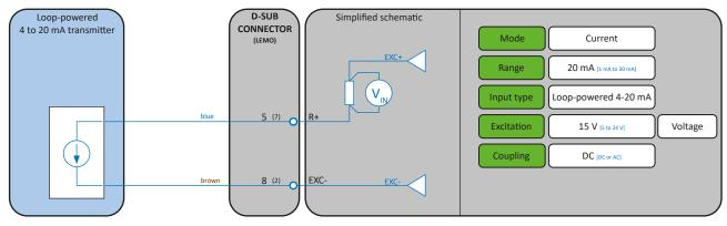
Fig. 52: Loop-powered 4 to 20 mA transmitter
