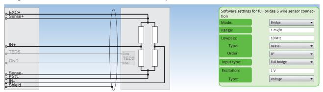
Fig. 80: Full bridge 6-wire sensor connection
