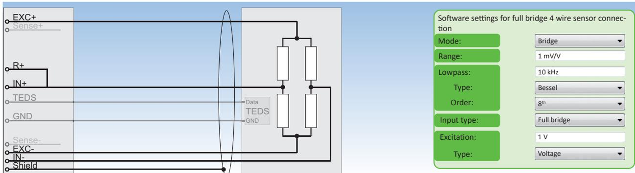
Fig. 62: Full bridge 4-wire sensor connection
