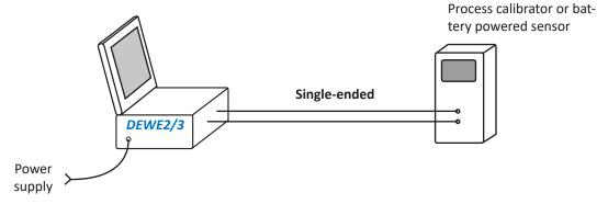
Fig. 123: Power supply / process calibrator or battery powered sensor
