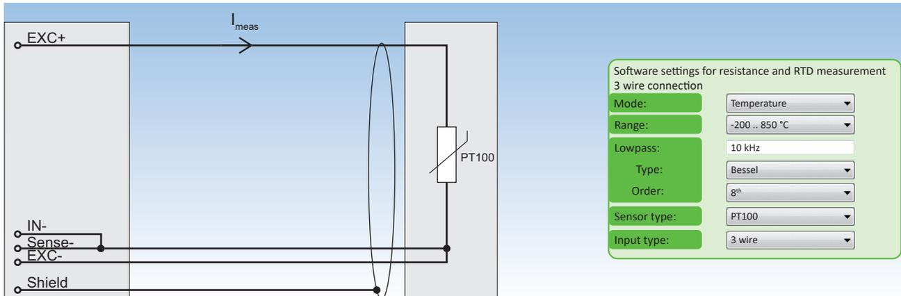
Fig. 68: Resistance and RTD measurement 3 wire connection
