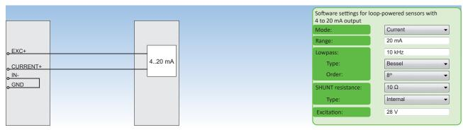
Fig. 31: Loop-powered sensors with 4 to 20 mA output
