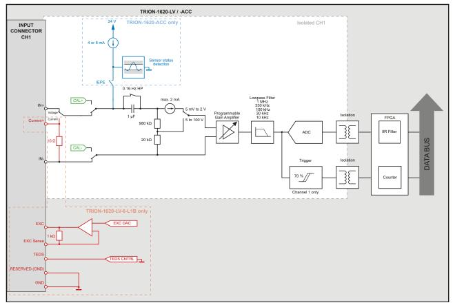
Fig. 26: Base block diagram of the TRION-1620-ACC/LV module
