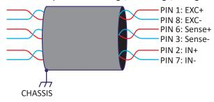
Fig. 73: Cables and shielding
