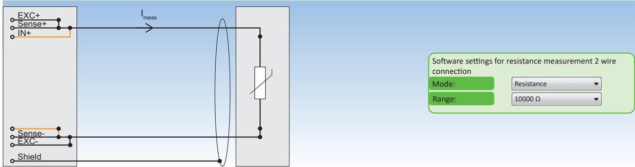
Fig. 127: Resistance and RTD measurement 2 wire connection
