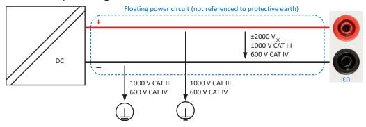
Fig. 136: Maximum input voltages
