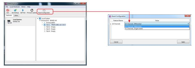
Fig. 100: Single-ended / differential mode
