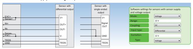
Fig. 105: Sensors with sensor supply and voltage output
