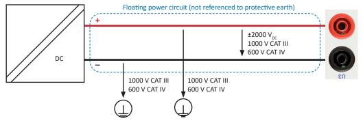
Fig. 135: Maximum input voltages
