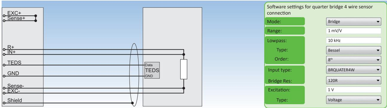
Fig. 66: Quarter bridge 4 wire sensor connection
