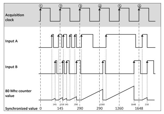
Fig. 197: Two Pulse Edge Separation Measurement
