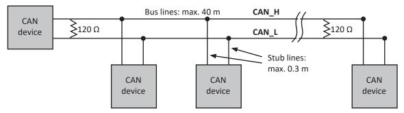
Fig. 198: High-speed CAN
