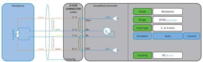
Fig. 66: Resistance measurement
