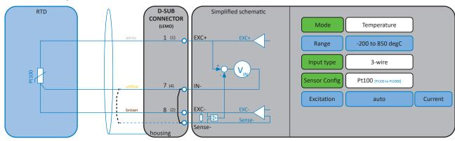
Fig. 68: RTD 3-wire temperature measurement
