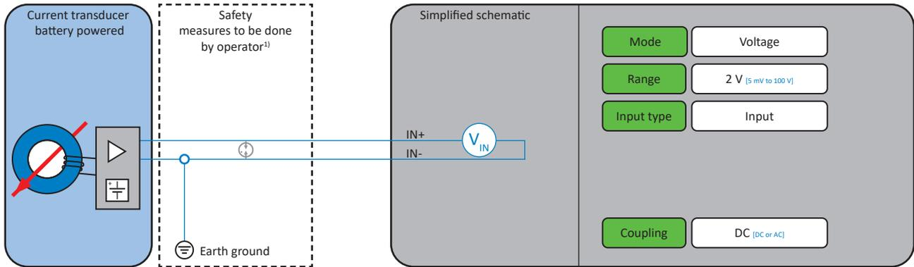
Fig. 86: Current transducer with voltage output
