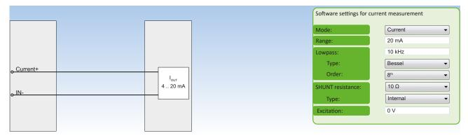
Fig. 29: Current measurement
