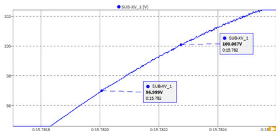
Fig. 232: TRION-SUB-XV auto ranging 100 V ↔ 1000 V switch over
