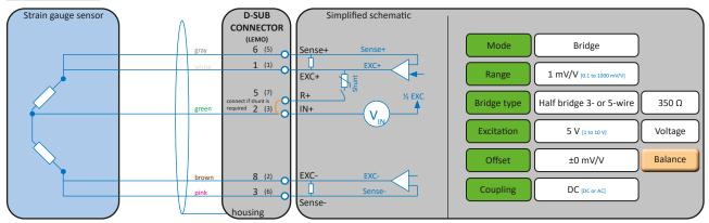
*Fig. 58: Half bridge 5-wire*
