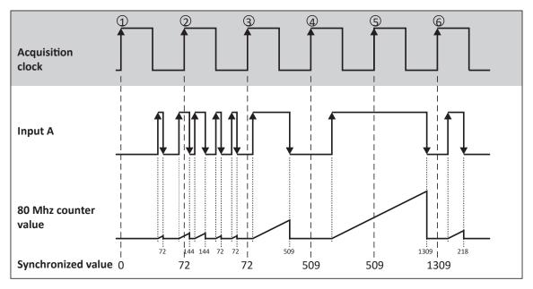
Fig. 189: Pulse width measurement
