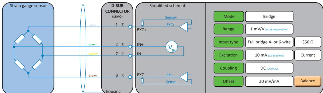
Fig. 37: Full bridge 4-wire with constant current excitation
