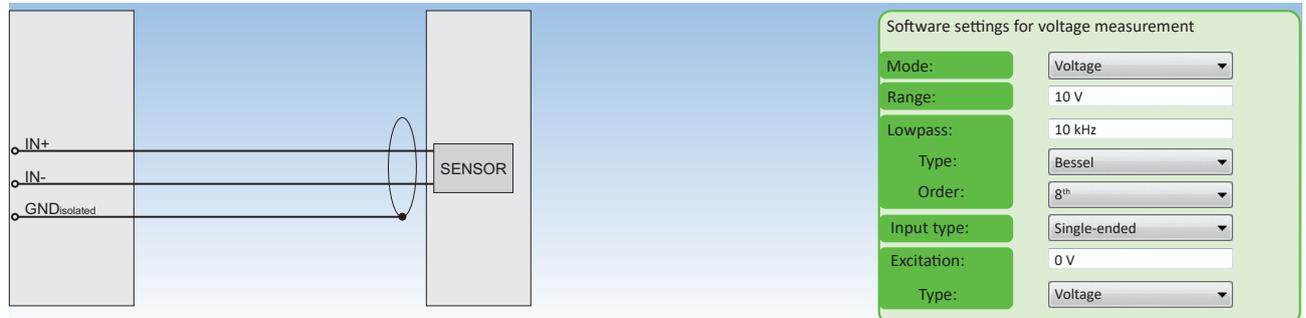
Fig. 58: Voltage measurement
