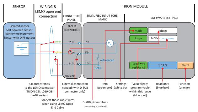
Fig. 47: Reading schematics
