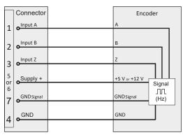
Fig. 167: Supplied sensor connection
