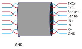
Fig. 116: Cables and shielding for full bridge, half bridge and voltage modes
