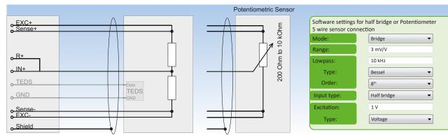
*Fig. 83: Half bridge or Potentiometer 5 wire sensor connection*
