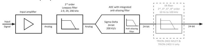
Fig. 7: TRION-2402 sample system architecture
