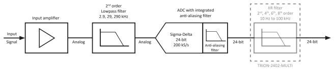
Fig. 7: TRION-2402 sample system architecture
