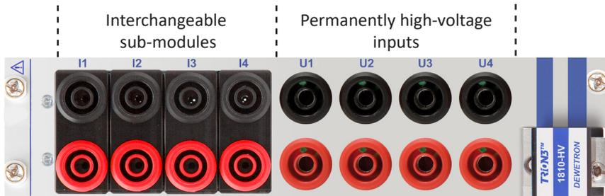
Fig. 142: Connection ports
