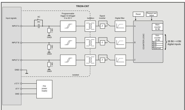
Fig. 190: Block diagram
