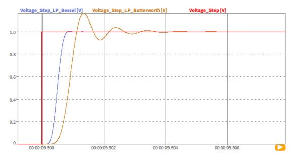
Fig. 140: Step response of filter with 1000 Hz cutoff frequency and 8th order.
