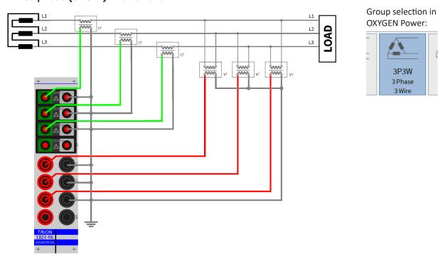
Fig. 146: Three phase (3P3W) with CT and VT
