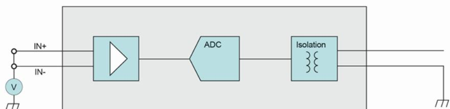
Fig. 245: Common mode voltage
