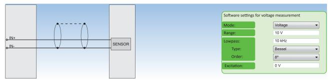
Fig. 37: Voltage measurement
