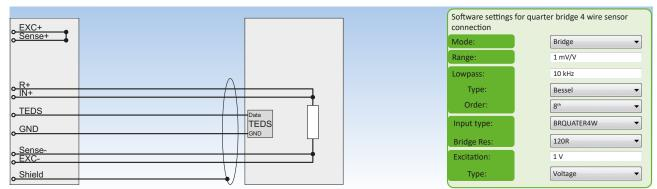
Fig. 86: Quarter bridge 4 wire sensor connection
