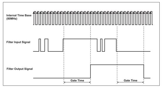
Fig. 193: Input signal with jitter
