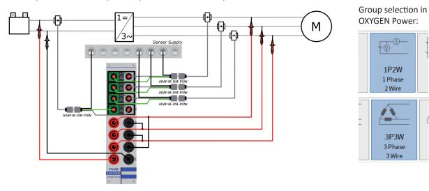
Fig. 149: Three phase and one phase (3P3W and 1P2W)
