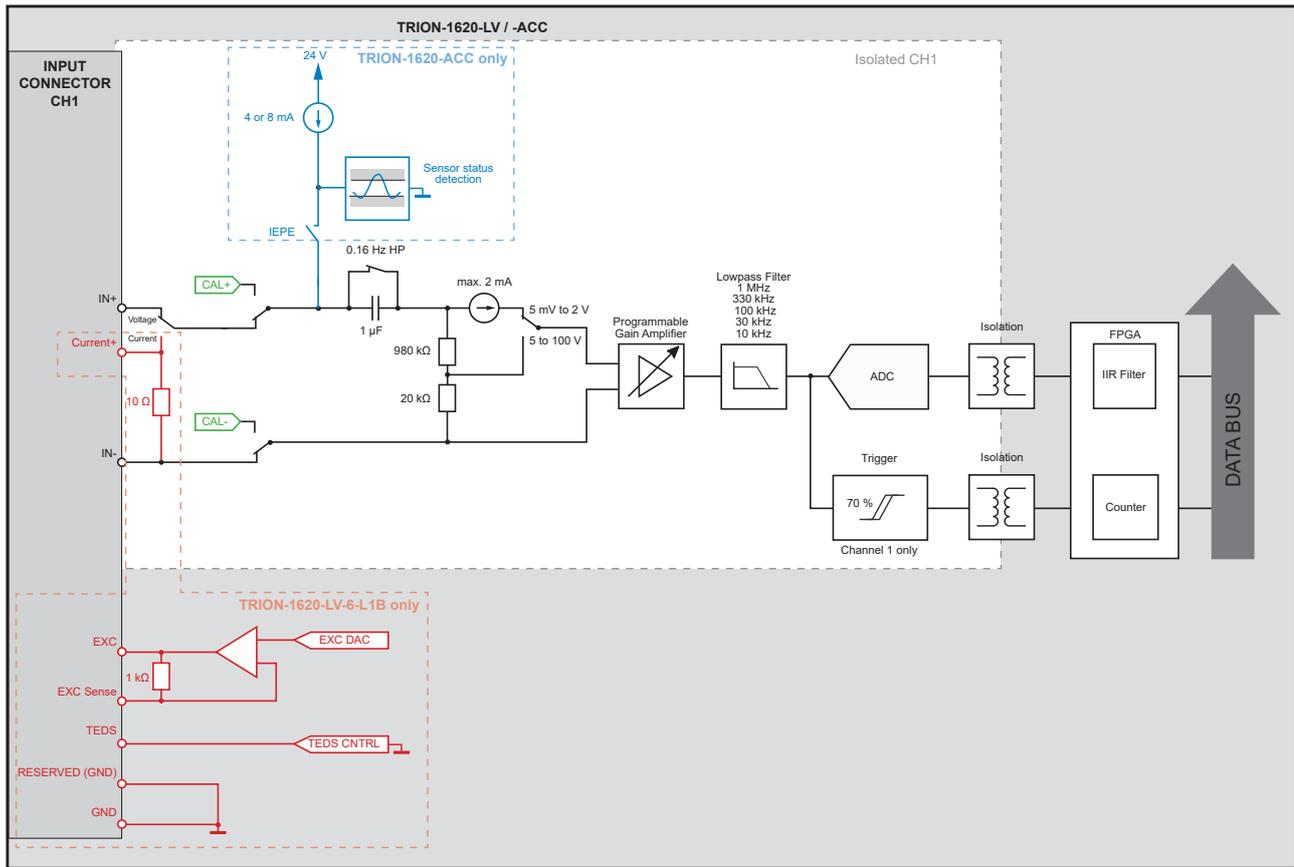
Fig. 92: Base block diagram of the TRION-1620-ACC/LV module
