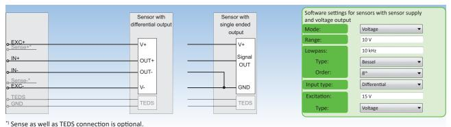
Fig. 79: Sensors with sensor supply and voltage output
