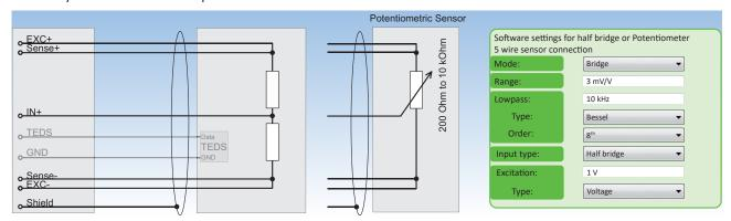
Fig. 82: Half bridge or Potentiometer 5 wire sensor connection
