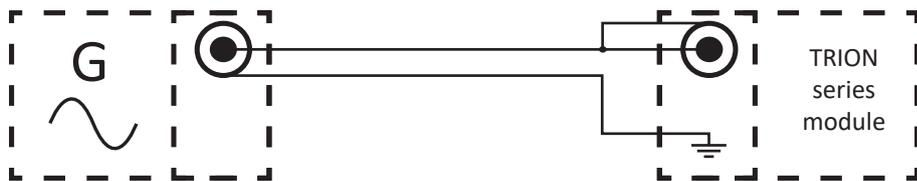
Fig. 239: Schematic circuit diagram of CMRR measurement
