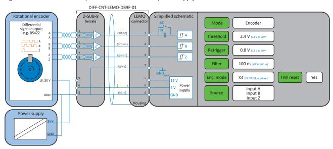
Fig. 188: Rotational encoder externally powered
