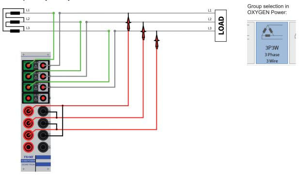
Fig. 143: Three phase (3P3W) without neutral line
