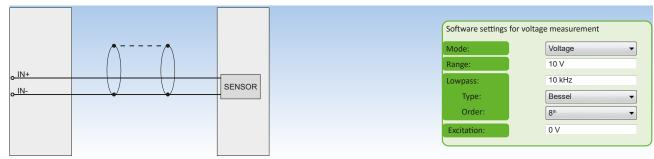
Fig. 37: Voltage measurement
