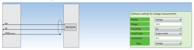
Fig. 105: Voltage measurement
