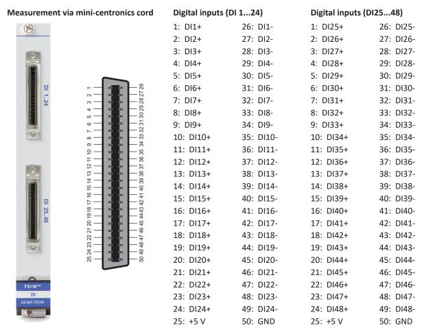
Fig. 216: 50-pin mini-centronics socket
