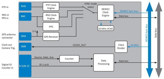
Fig. 170: Signal routing
