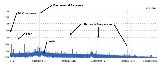
Fig. 205: FFT chart of TRION-1620-ACC
