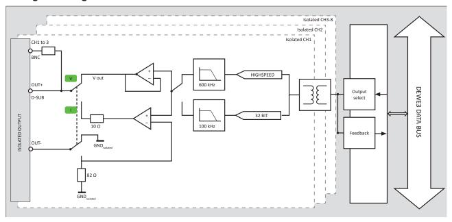
Fig. 163: Analog block diagram
