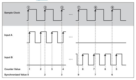
Fig. 202: A-Up/B-down encoder
