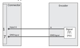
Fig. 181: Non-supplied sensor connection
