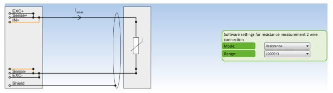
Fig. 114: Resistance and RTD measurement 2 wire connection
