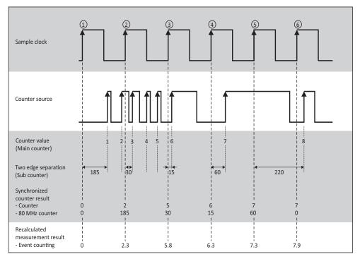
Fig. 196: Frequency measurement
