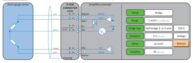
Fig. 58: Half bridge 5-wire
