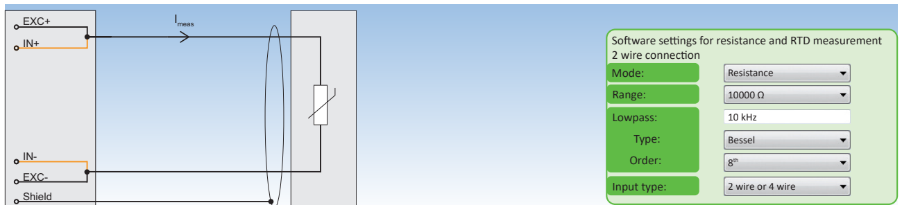
Fig. 87: Resistance and RTD measurement 2 wire connection
