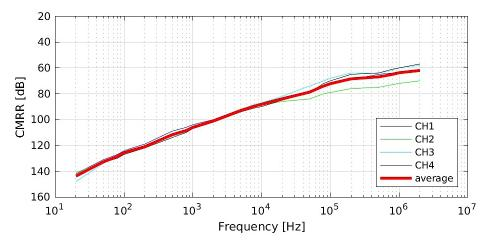
Fig. 228: CMRR over frequency response of a TRION-1820-POWER-4 (V inputs) (not a directly measured FFT chart)
