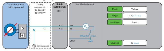
Fig. 51: Current transducer with voltage output
