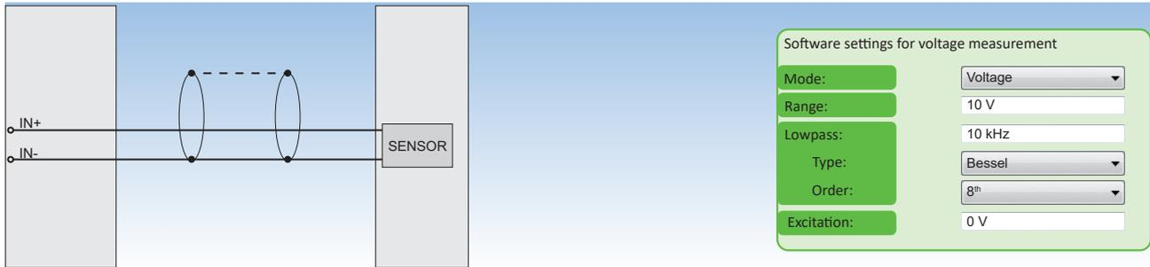
Fig. 93: Voltage measurement
