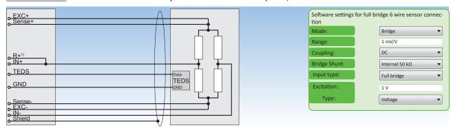
Fig. 108: Full bridge 6-wire sensor connection
