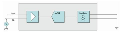
Fig. 229: Isolation voltage
