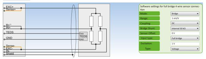
Fig. 109: Full bridge 4-wire sensor connection
