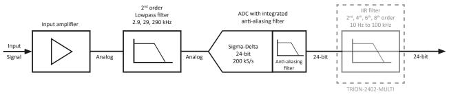
Fig. 7: TRION-2402 sample system architecture
