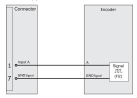
Fig. 168: Non-supplied sensor connection
