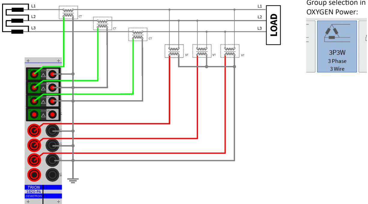
Fig. 160: Three phase (3P3W) with CT and VT
