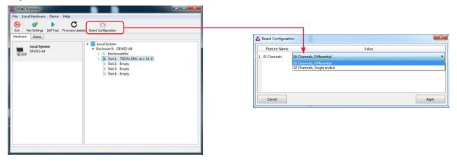
Fig. 99: Single-ended / differential mode
