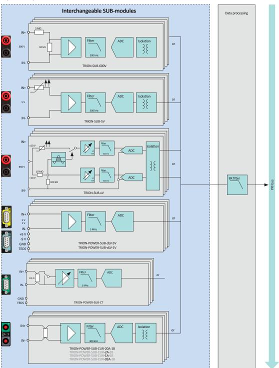
Fig. 163: Block diagram
