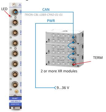
Fig. 91: Connecting XR modules to the TRION-2402-MULTI module
