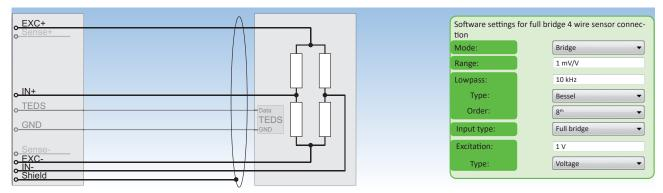
Fig. 81: Full bridge 4-wire sensor connection
