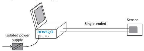
Fig. 122: Isolated power supply/sensor
