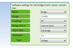
Fig. 108: Full bridge 6-wire sensor connection
