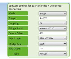
Fig. 113: Quarter bridge 4 wire sensor connection
