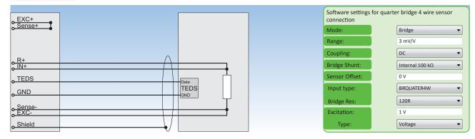
Fig. 112: Quarter bridge 4 wire sensor connection
