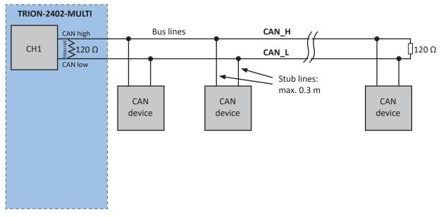
Fig. 90: CAN bus connection
