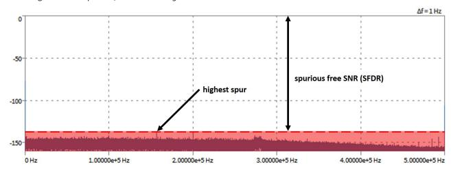
Fig. 207: SFDR in a FFT chart without input signal (DEWETRON)
