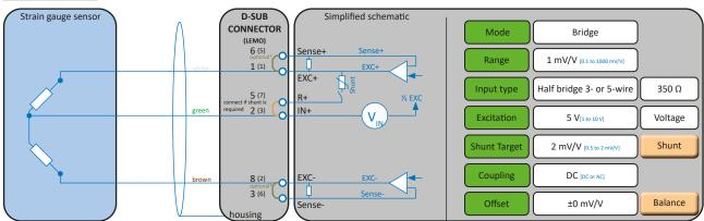
Fig. 60: Half bridge 3-wire
