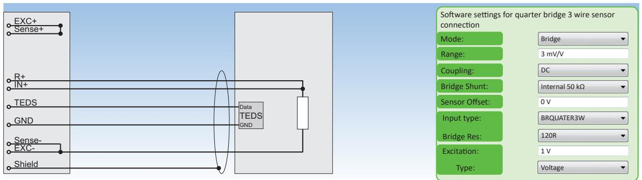
Fig. 125: Quarter bridge 3 wire sensor connection
