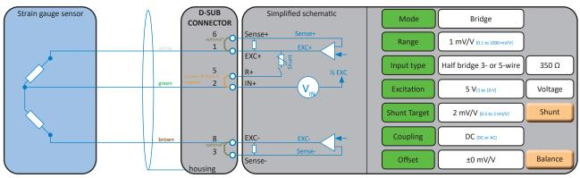
Fig. 59: Half bridge 3-wire
