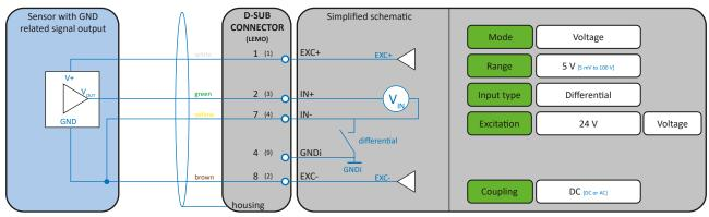
Fig. 50: Single-ended sensor powered by the TRION module
