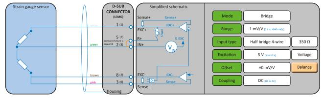
Fig. 59: Half bridge 4-wire
