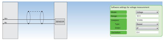
Fig. 37: Voltage measurement
