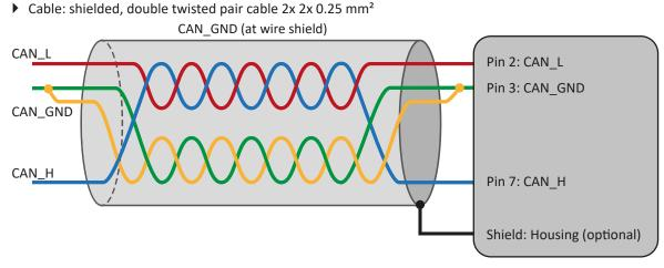
Fig. 210: Cabling for heavy industrial environment
