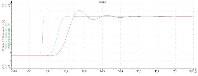
Fig. 12: Step response TRION(3)-18xx-MULTI series
