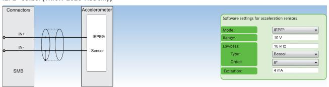
Fig. 32: IEPE® sensor (TRION-1620-ACC only)
