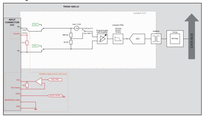
Fig. 36: Base block diagram of the TRION-1603-LV module
