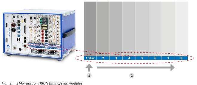
**1.** TRION(3) system timing slot
