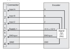
Fig. 166: Supplied sensor connection
