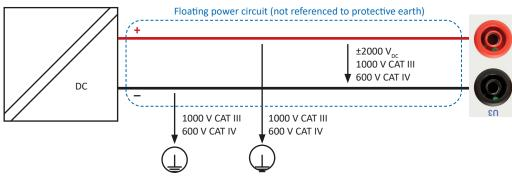
Fig. 136: Maximum input voltages
