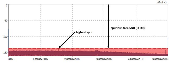
Fig. 223: SFDR in a FFT chart without input signal (DEWETRON)
