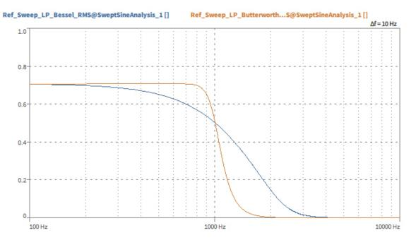
Fig. 142: Frequency response of filter with 1000 Hz cutoff frequency and 8th order
