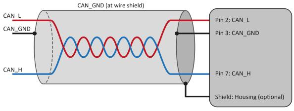
Fig. 209: Cabling for light industrial environment
