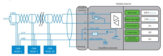
Fig. 207: Connecting sensors directly supplied by TRION3-CAN-FD
