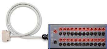
24 channel break-out box with 4 mm banana jacks. 1 m cable, terminated with 50-pin mini-centronics plug.
