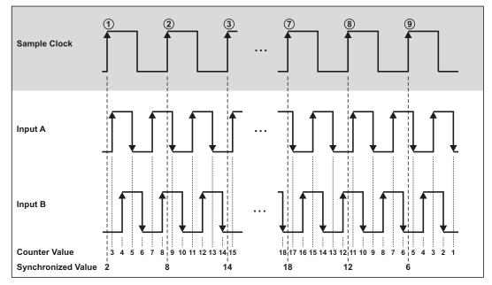
Fig. 200: Quadrature Encoder X4 Mode
