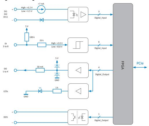
Fig. 43: Digital block diagram
