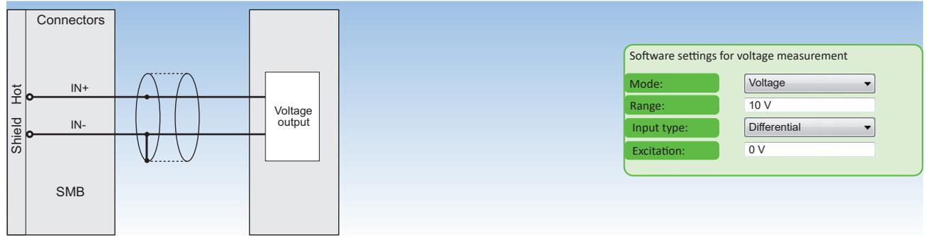
Fig. 139: Voltage measurement
