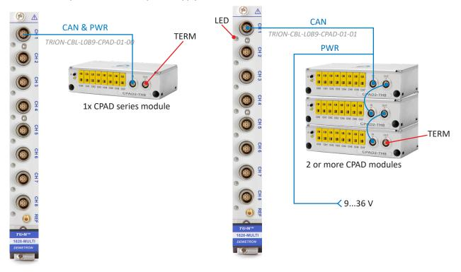
Fig. 90: Connecting CPADs to the TRION-2402-MULTI module
