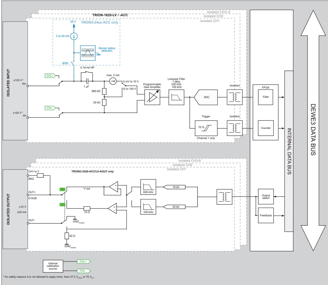
Fig. 80: Analog block diagram
