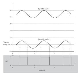
Fig. 183: Programmable trigger level
