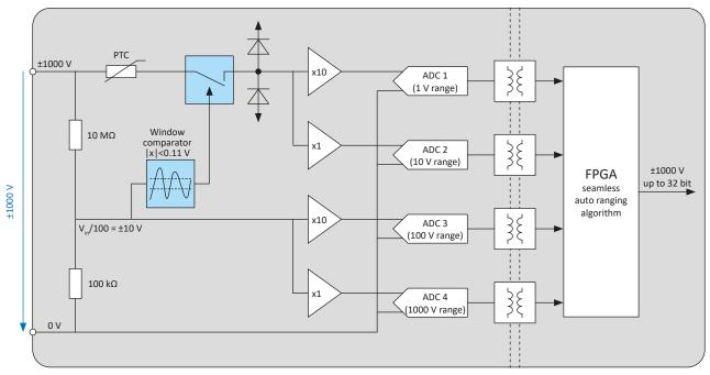
Fig. 218: Block diagram TRION-SUB-XV
