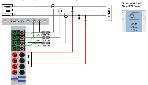
Fig. 144: Three phase (3P3W) without neutral line, using current output transducer
