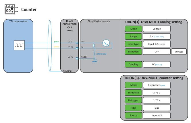
Fig. 69: Counter measurement
