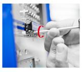
4. Pull down the injector/ejector handle or use the TRION extraction tool to release the module.
