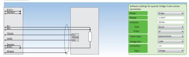
Fig. 85: Quarter bridge 3 wire sensor connection
