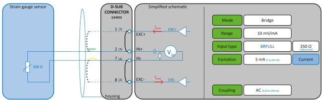
Fig. 64: Strain measurement with constant-current supply and AC coupling"
