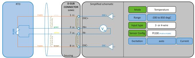
Fig. 67: RTD 2- and 4-wire temperature measurement
