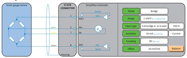
Fig. 56: Full bridge 4-wire with constant current excitation
