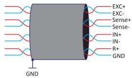
Fig. 115: Cables and shielding for full bridge, half bridge and voltage modes
