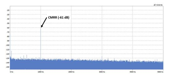
Fig. 211: Measurement of CMRR in FFT chart of TRION-1620-ACC (>2 V range @ 1 kHz)
