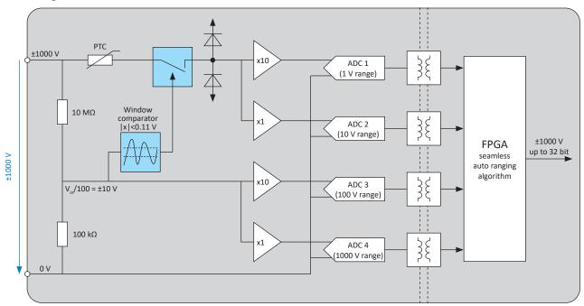
Fig. 218: Block diagram TRION-SUB-XV
