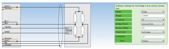
Fig. 108: Full bridge 4-wire sensor connection
