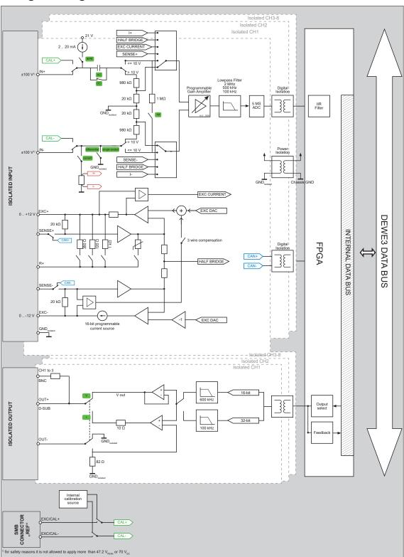
Fig. 44: Analog block diagram
