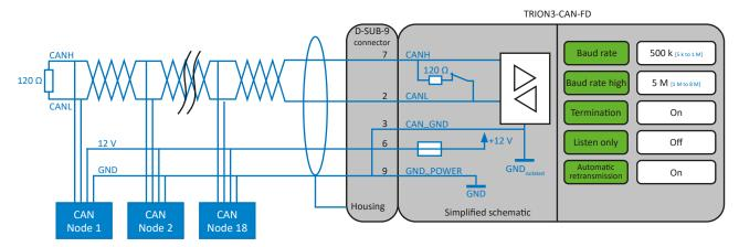
Fig. 207: Connecting sensors directly supplied by TRION3-CAN-FD
