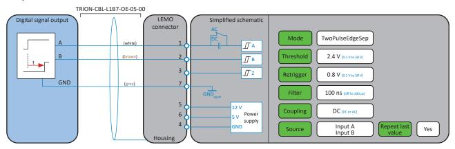
Fig. 183: Two pulse edge separation
