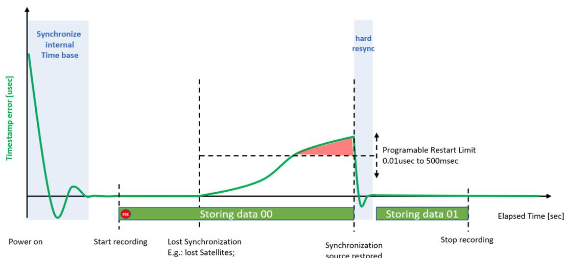
Fig. 188: Forced restart after restored synchronization
