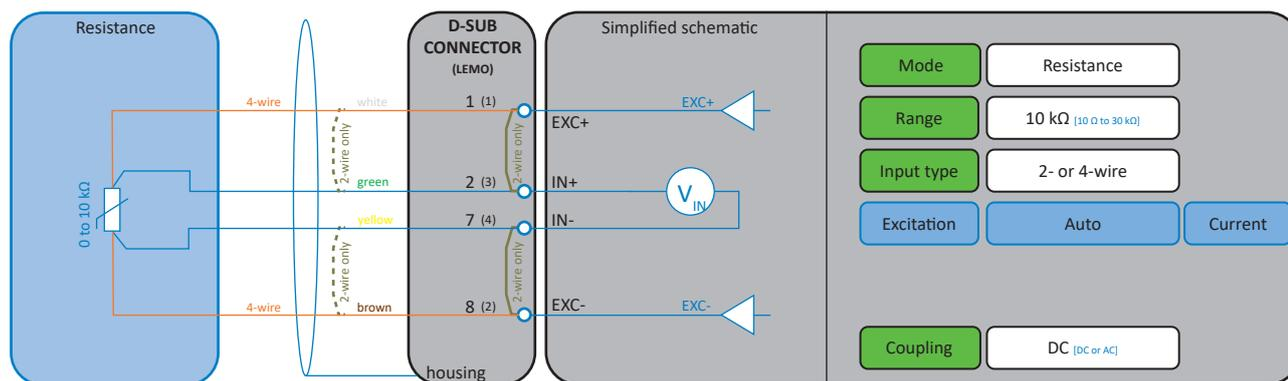
Fig. 46: Resistance measurement
