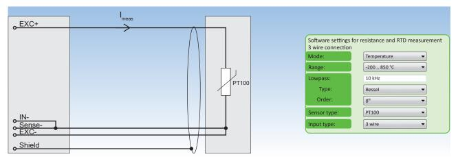
Fig. 87: Resistance and RTD measurement 3 wire connection
