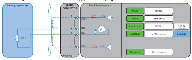
Fig. 63: Quarter bridge 2-wire with constant current supply and AC coupling
