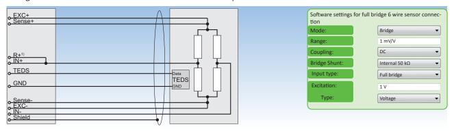
Fig. 107: Full bridge 6-wire sensor connection
