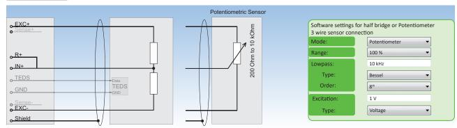
Fig. 84: Half bridge or Potentiometer 3 wire sensor connection
