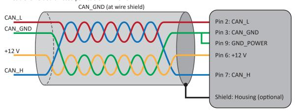
Fig. 211: Cabling for sensors with power supply
