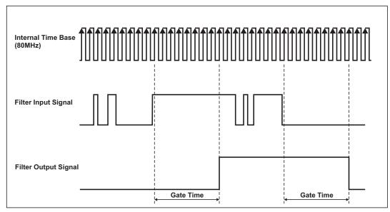
Fig. 185: Input signal with jitter
