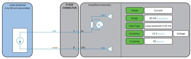
Fig. 51: Loop-powered 4 to 20 mA transmitter
