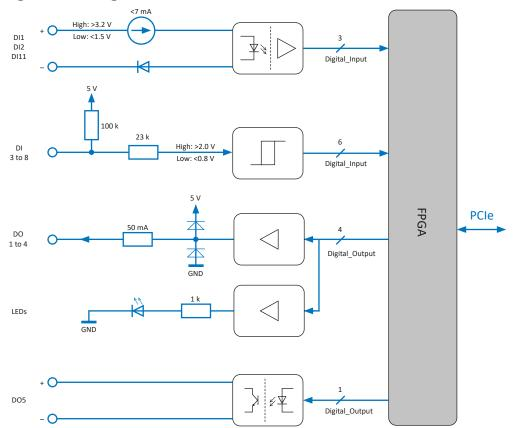
Fig. 43: Digital block diagram
