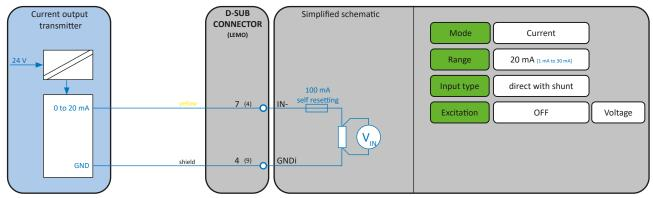
Fig. 53: Current measurement (with externally powered transmitter)
