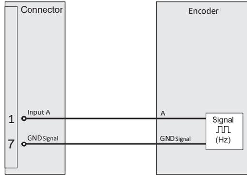
Fig. 181: Non-supplied sensor connection
