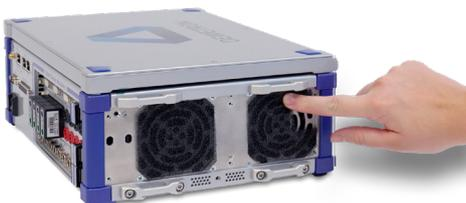
7. Remount the covering plate by tightening the 6 screws using a TORX T10 screwdriver.
