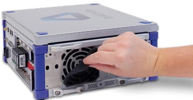
5. Clean the filterpads with a dry velocity stream of air.
