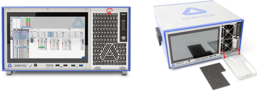
Fig. 42: Filter pad cleaning
