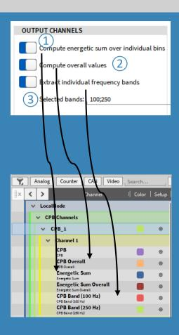
The actual CPB spectrum (changing in time) is calculated per default. The channel name is *CPB*
