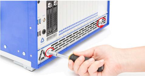
3. Grab both screws and firmly pull out the fan cartridge. With a slight downward movement the cartridge can be fully released.
