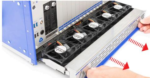
4. To remove the protective grille flip over the cartridge.
