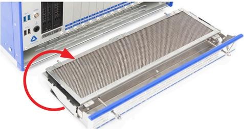
5. Loosen the screws on both sides with a TORX T8 screwdriver.
