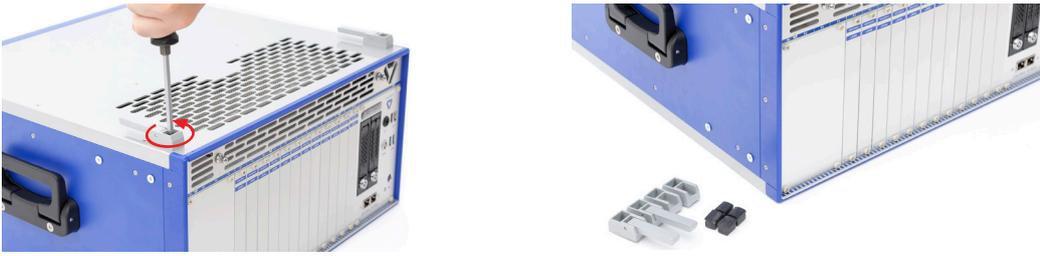
The feet are now removed and the device is ready for installation in a control cabinet.
