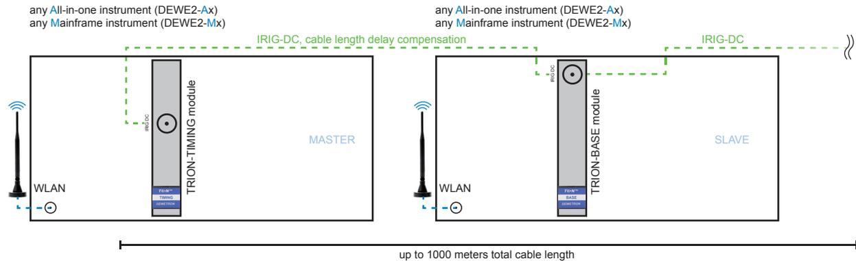
Usually the connection of the instruments is done via WLAN. If no WLAN option is available with your system, the connection is done via ethernet (CATVI) cable.
