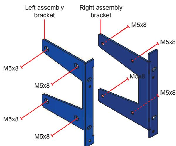
**WARNING:** *When installing the 19" mounting brackets, the maximum length for screws is 8 mm! If any screw get lost replace it with M5x8 countersunk head screw only. Otherwise the TRION™ series cards or the powersupply could get damaged!*
