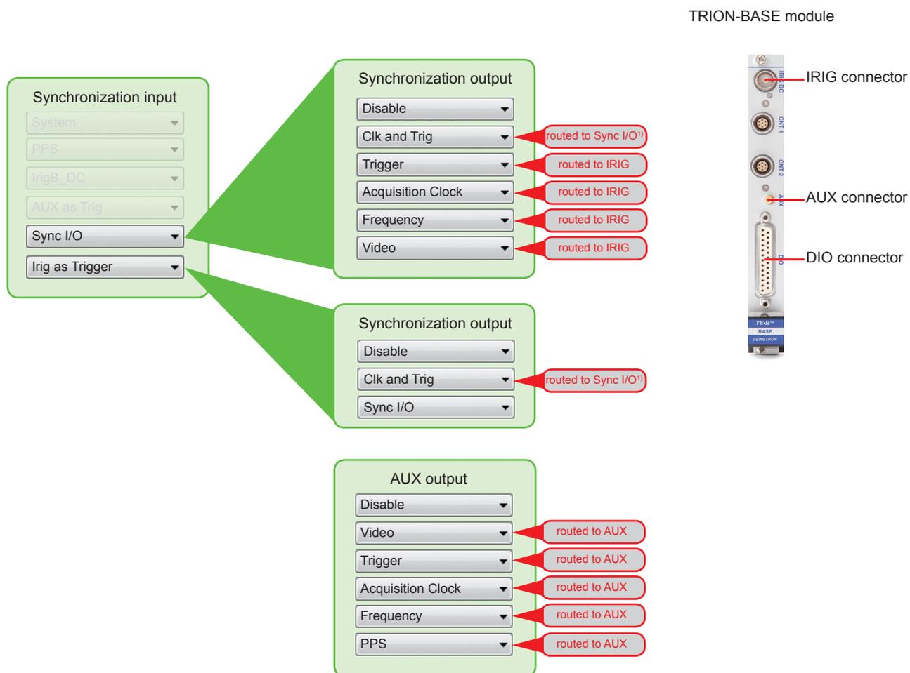
1) When using 'Sync I/O' or 'Irig as Trigger' for synchronization input and 'Clk and Trig' as synchronization output, DEWESoft 7.x displays 'routed to Sync I/O'. It is routed to the **DIO connector** of the **TRION-TIMING** module. **This is an error in DEWESoft 7.x!**
