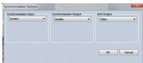
Some TRION™ series modules (TRION-TIMING /-BASE) support an additional SMB connector, labelled "AUX" on the front panel. It is possible to route some signals to SMB connector, e.g. Video, Trigger, Acquisition clock, Frequency or PPS.
