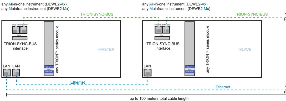
The instruments are connected via standard Ethernet (CATVI) cable or via WLAN, if installed.
