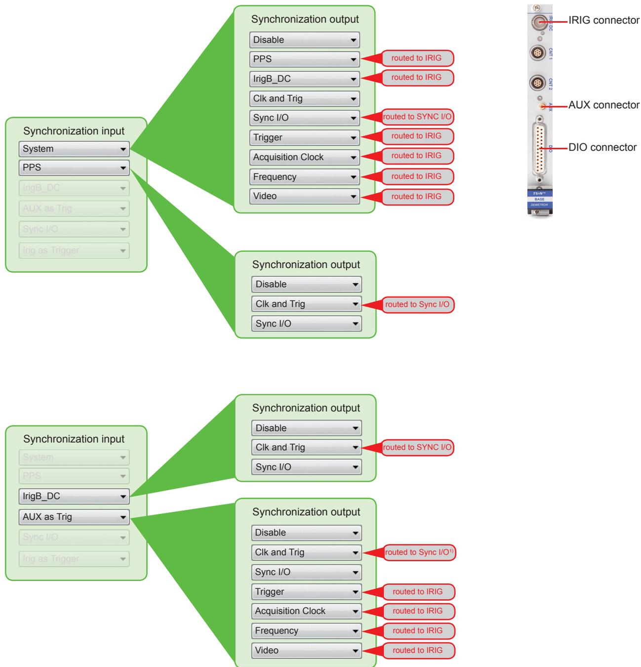
1) When using 'AUX as Trigger' for synchronization input and 'Clk and Trig' as synchronization output, DEWESoft 7.x displays 'routed to Sync I/O'. It is routed to the **DIO connector** of the **TRION-TIMING module**. This is an error in DEWESoft 7.x!
