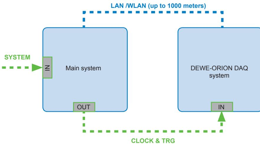
When choosing "CLOCK & TRG" as synchronization output at the master system, the signals are routed automatically to the "DIO" connector. Please refer to chapter "2.9 Synchronization options in DEWESoft" for detailed information
