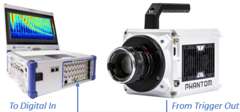
Fig. 7.160: Recording start of DAQ system triggered by camera
