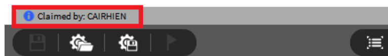
Fig. 15.13: Claimed information on the Slave device. In this case, the Master device is named CAIRHIEN
