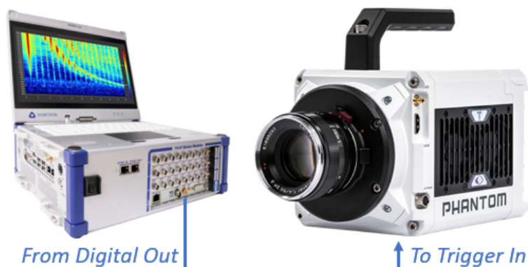
Fig. 7.164: Recording start of camera triggered by DAQ system
