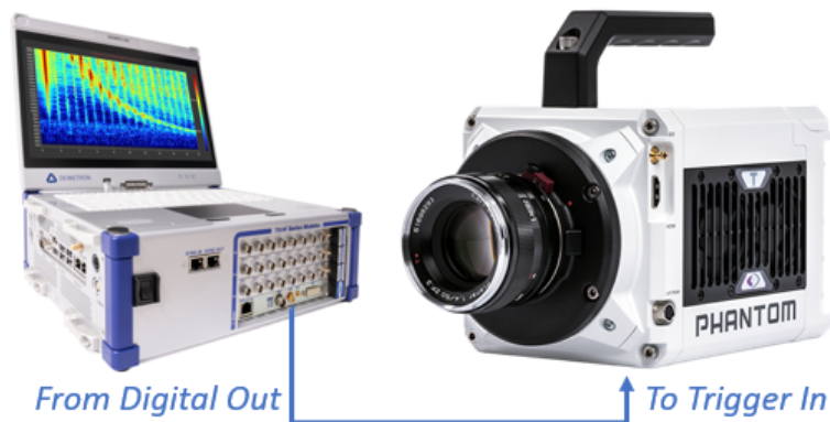
Fig. 7.152: Recording start of camera triggered by DAQ system
