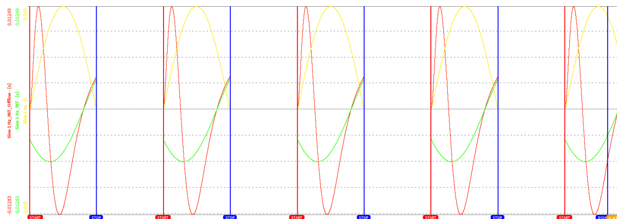
Fig. 7.175: Deviation of Offline and Online Filter channels in case of Event based Waveform recording
