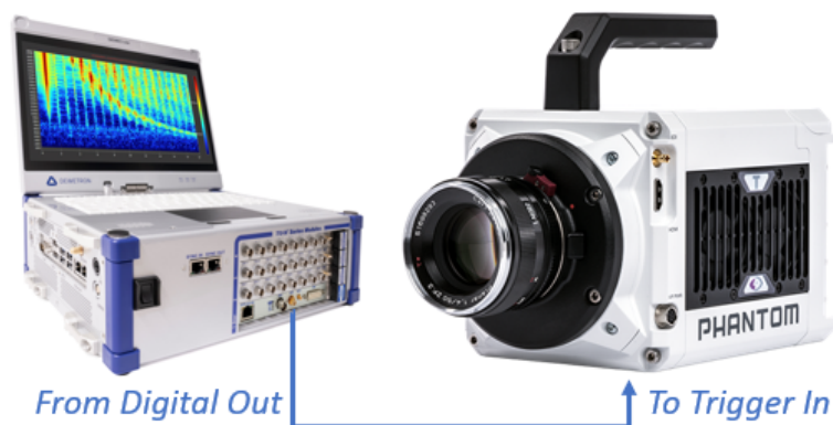
Fig. 7.161: Recording start of camera triggered by DAQ system
