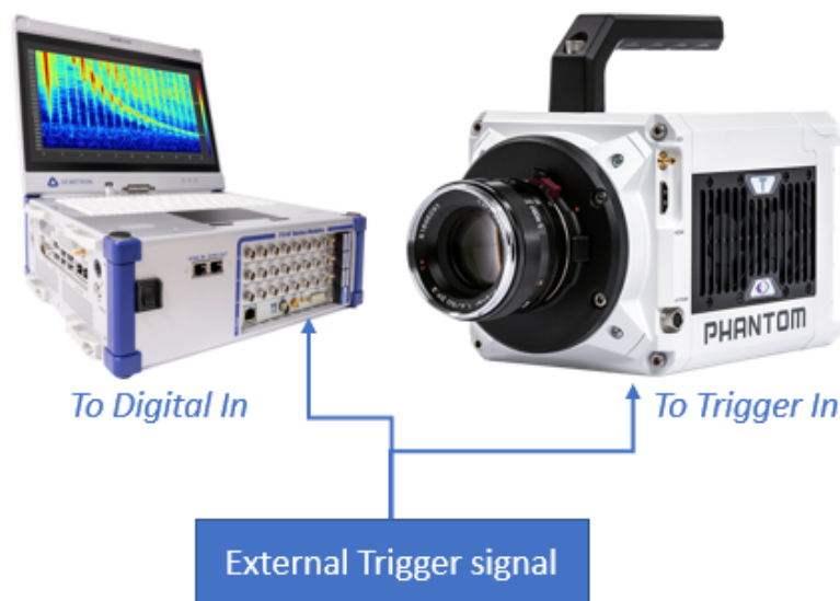
Fig. 7.164: Recording start of DAQ system and camera triggered by external signal
