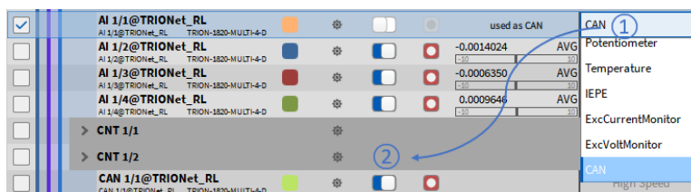
Fig. 7.189: Using the CAN port of a TRION-MULTI board
