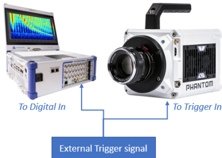
Fig. 7.159: Recording start of DAQ system and camera triggered by external signal
