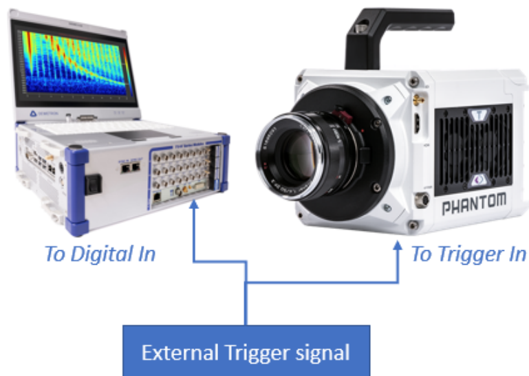
Fig. 7.162: Recording start of DAQ system and camera triggered by external signal
