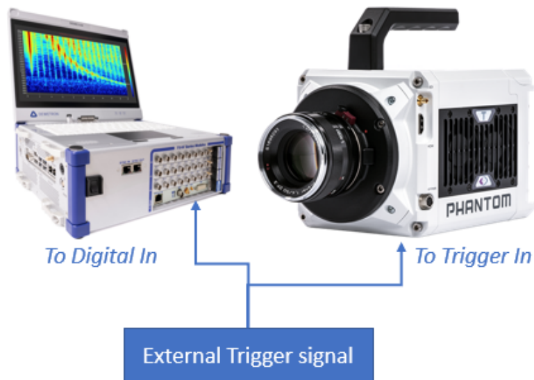
Fig. 7.150: Recording start of DAQ system and camera triggered by external signal
