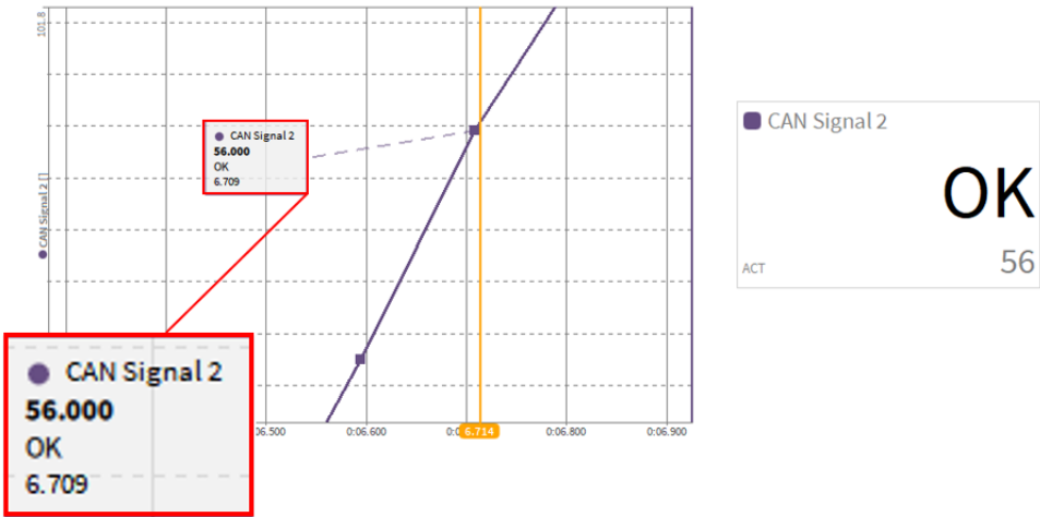
Fig. 7.43: Enum Scaling - display in the digital instrument and as label in the recorder
