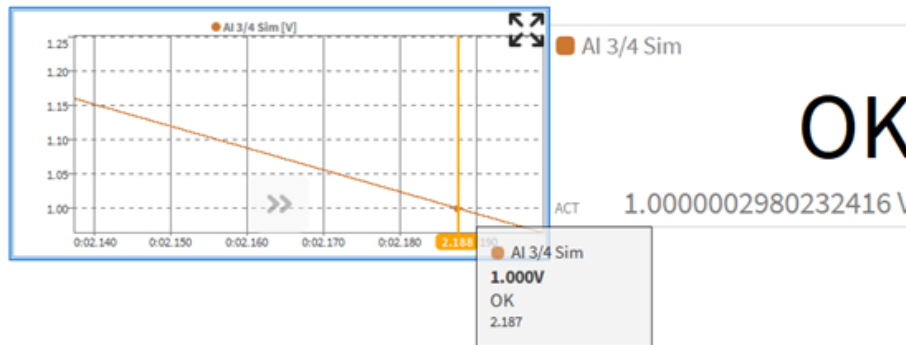
Fig. 7.43: Enum Scaling - display in the digital instrument and as label in the recorder
