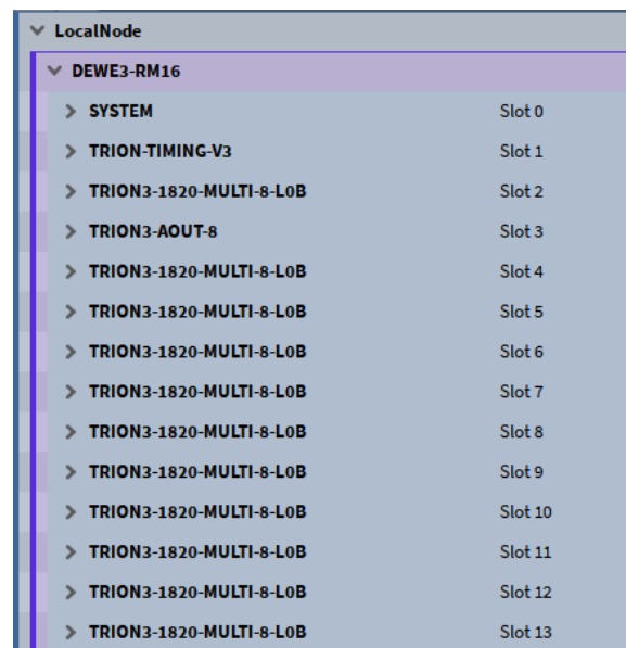
Fig. 7.4: Slot numbering with folded modules
