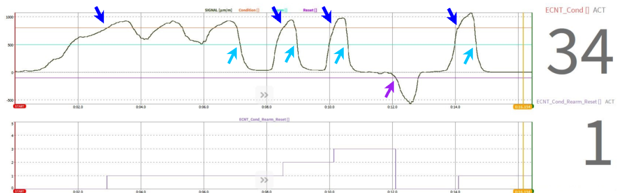
Fig. 7.55: ECNT-function with Condition, Rearm and Reset
