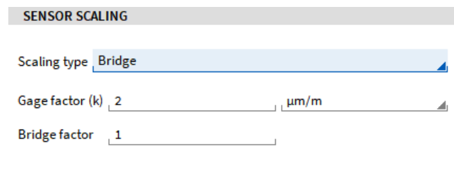
Fig. 7.26: Scaling setting for bridge mode
