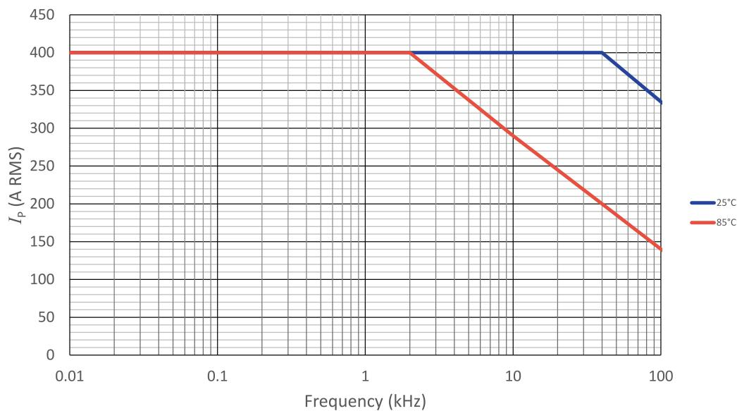
Figure 6: Derating curve
