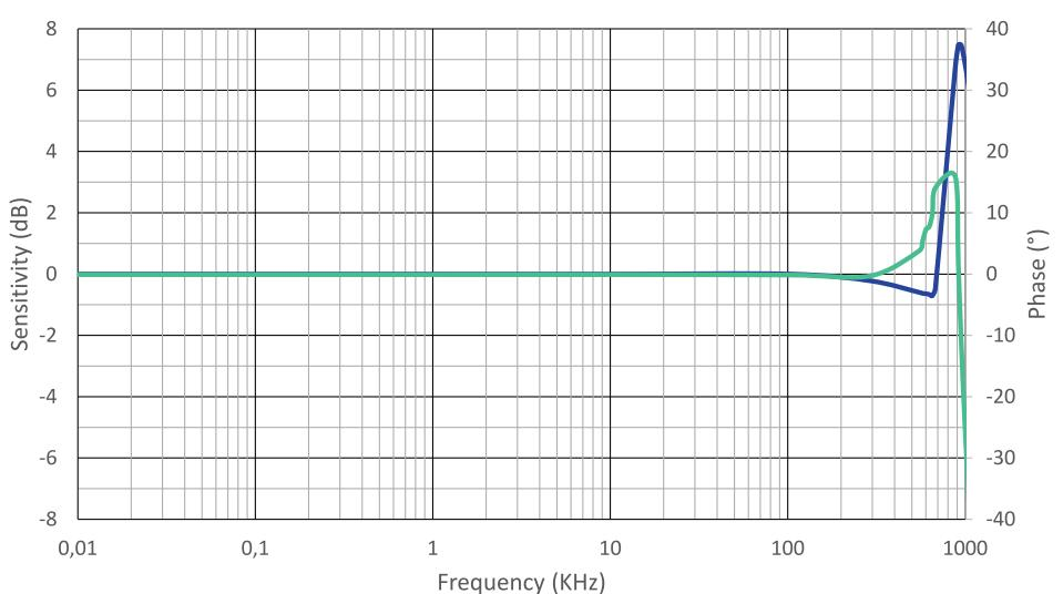
Figure 5: Typical transducer bandwidth response at 25 °C under 1.5 Ω
