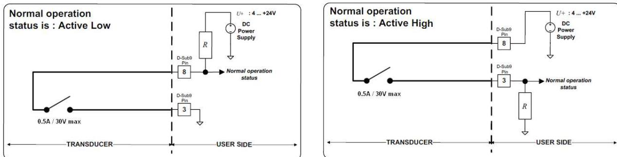
The measuring can resume when the primary current returns in the measuring range (see measuring range figures in [page 7](#)). Then the signal normal operation status switches to GND and the green LED indicator (normal operation status) is closed.
