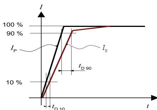
Figure 9:  $t_{D10}$  (delay time @ 10 %) and  $t_{D90}$  (delay time)
