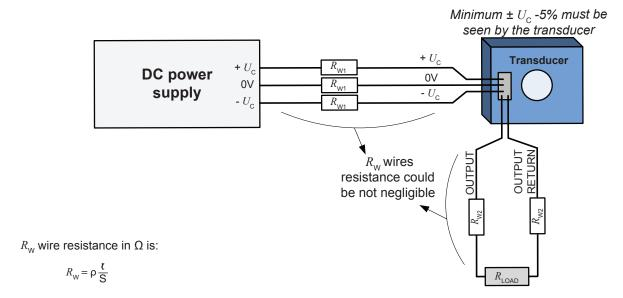
S: Cross section of wire in m<sup>2</sup>
