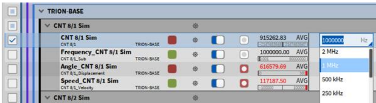
Figure 2-2: Changing the sample rate of the counter channel
