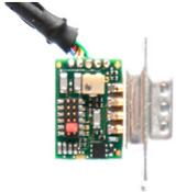
4. Connect the MSI2-LVDT to the measurement system with an extension cable.
