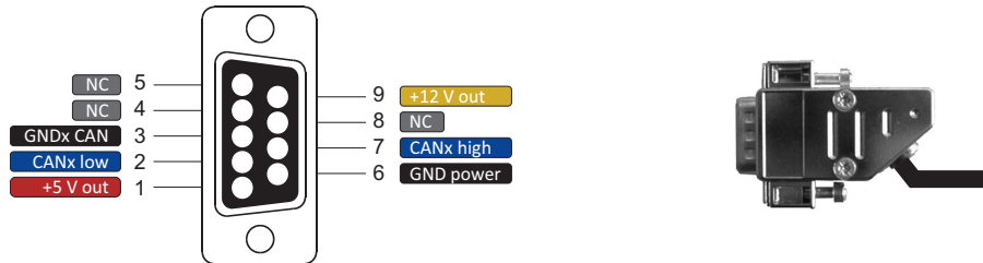
Fig. 14: D-SUB-9 CAN connector pin assignment
