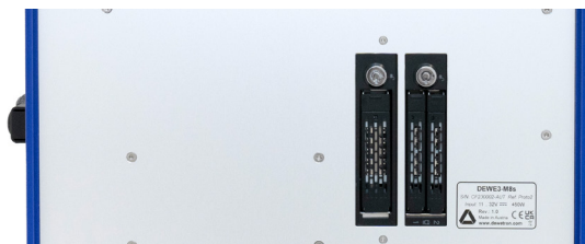
Fig. 18: Drive bays on backside
