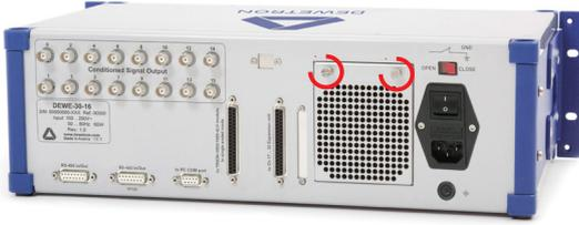
3. Remove the covering plate and the filter pads.
