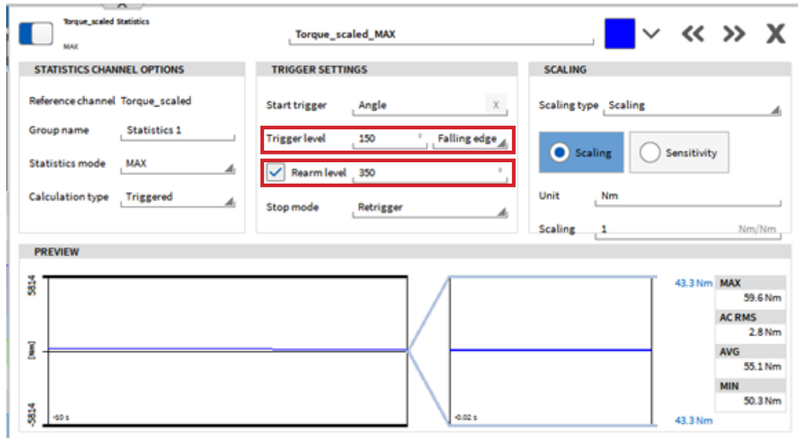
Fig. 6: Triggered statistics for torque ripple calculation.
