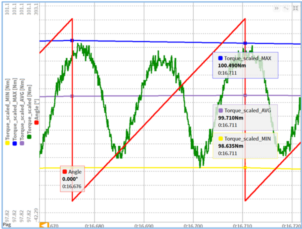
Fig. 5: Detail view of torque over one revolution.
