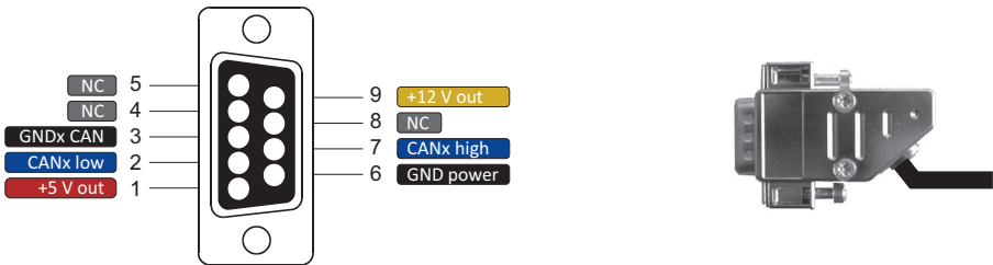
Fig. 9: D-SUB-9 CAN connector pin assignment
