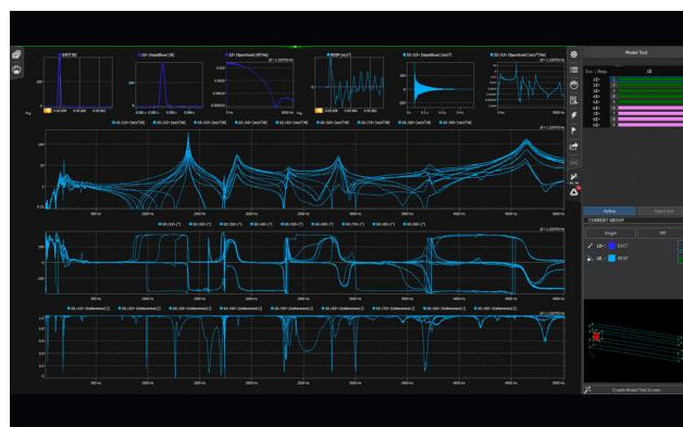
With OXYGEN's Modal Test option, analyze the frequency characteristics of a mechanical structure to determine resonances and damping.
