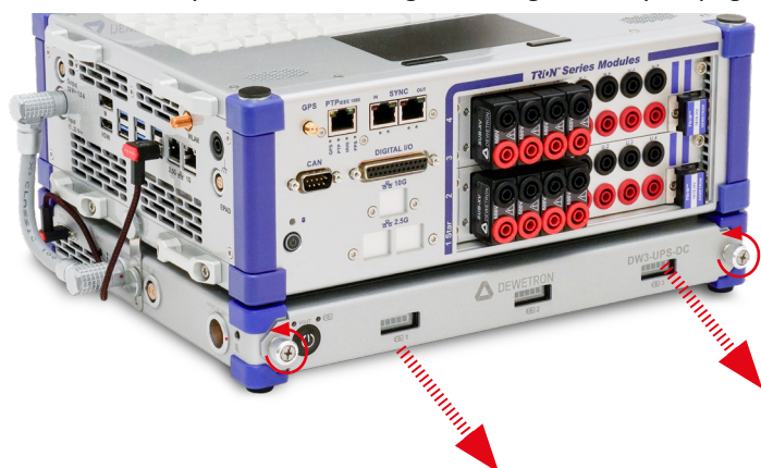
Fig. 8: Knurled-head screws for battery cover
