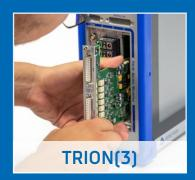
USER-EXCHANGEABLE TRION(3) MODULES FOR ALL INPUT SIGNALS: UP TO 10 MS/S
